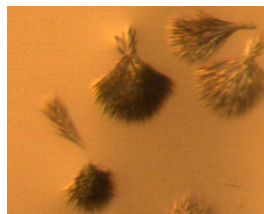
Figure 29: Urchin-like crystals obtained for nucleotide free complex \Delta 17\text{Arf1-BRAG2}^{\text{Sec7-PH}} . Obtained with proplex screen (Qiagen) in condition 0.1 M KCl, 0.1 M Tris pH 8, 15% PEG 2000 MME.
