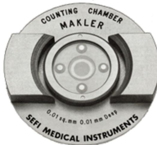
Fig. 1 Makler counting chamber, metallic base tool to evaluate sperm amount. (Makler, 1980)
