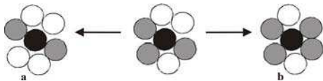
FIGURE 4. Schematic of the sound-induced change in Z : decrease via acoustic fluidization (a) and increase via particle buckling (b). The associated packing density remains unchanged in both cases. The spheres in grey are under stress associated with the force chains.
