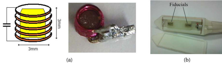
Figure 1.11: Passive tracking using resonant micro-coils. (a): Schematic (left) and photo (right) of a resonant micro-coil. (b): Endorectal device for prostate biopsies equipped with two micro-coils. Reprinted from [RME + 08].
