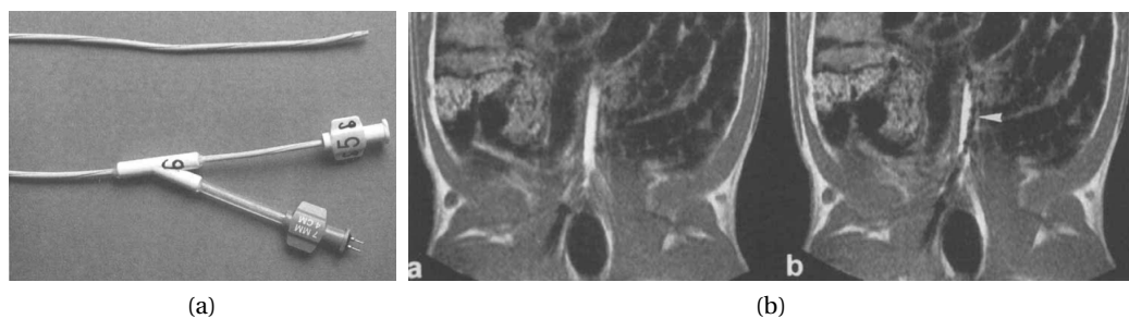
Figure 1.12: Catheter tracking with a wire loop through which current is led. (a): The conducting wire is wound helically around the catheter. (b): Comparison of the catheter visibility in a pig study without current (left) and with 150 mA (right). Reprinted from [GAB + 97].
