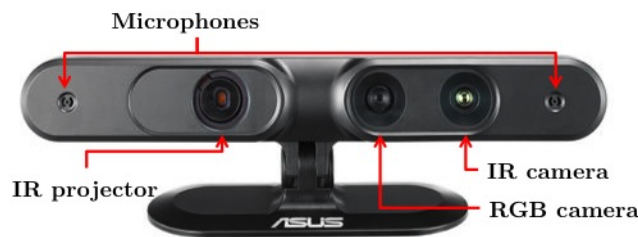
Figure 4.2: RGB-D sensor Asus Xtion Pro Live with infrared projector, RGB camera, infrared camera and microphones (reprinted from [htt13c]).
