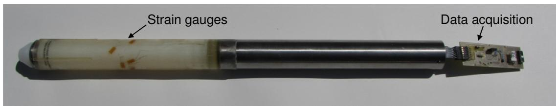
Figure 2.12: STT cell and data acquisition unit.
