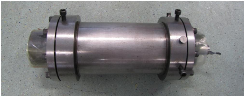
Figure 2.16: Biaxial test chamber with the core.
