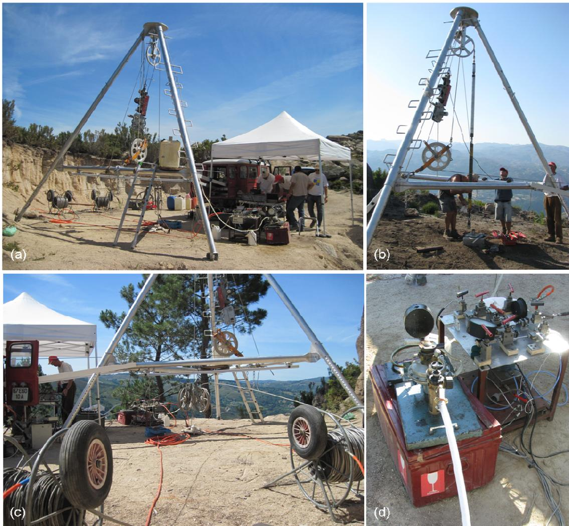
Figure 2.9: Hydraulic tests performed at the Paradela II site: (a) general view of the testing scheme, (b) downward movement of the upper packer, (c) downward movement of the system with the coiled tubing and (d) hydraulic pump.
