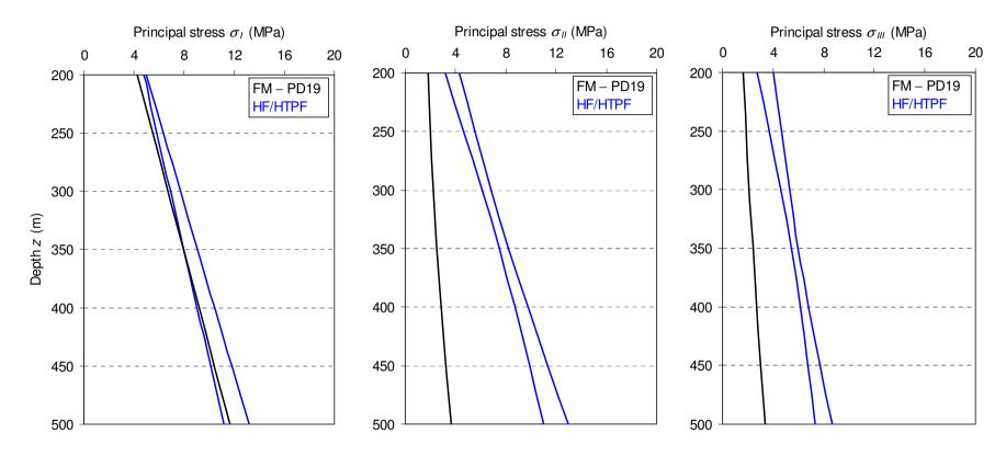
Figure 3.12: Variation of the magnitude of the principal stresses ( $\sigma_l$ ,  $\sigma_{ll}$ ,  $\sigma_{lll}$ ) obtained from the inversion of the hydraulic data (HF/HTPF) and with the FLAC3D model (FM) run with gravity loading only as functions of depth
