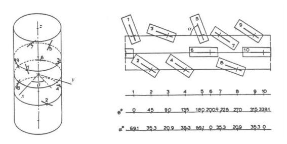
Figure 2.13: Orientation of the strain gauges in the STT cell.
