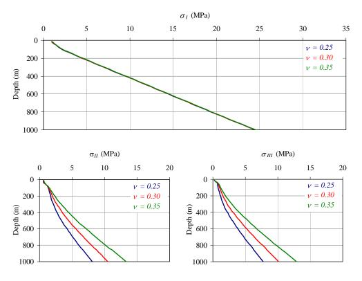
Figure 13. Comparison of the magnitudes of the principal stresses obtained at the location of the borehole PD19 for the gravity loading, with the values of 0.25, 0.30 and 0.35 for the Poisson's ratio.
