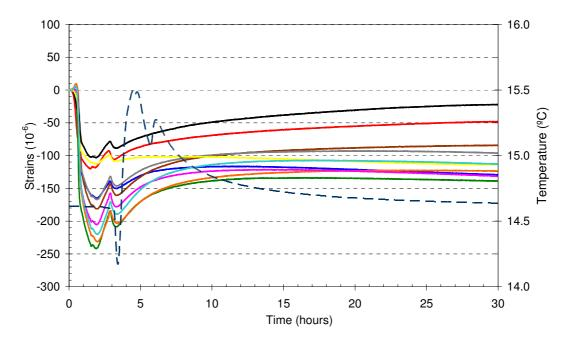
Figure 2.15: Record of strains and temperature as a function of time through an overcoring test.
