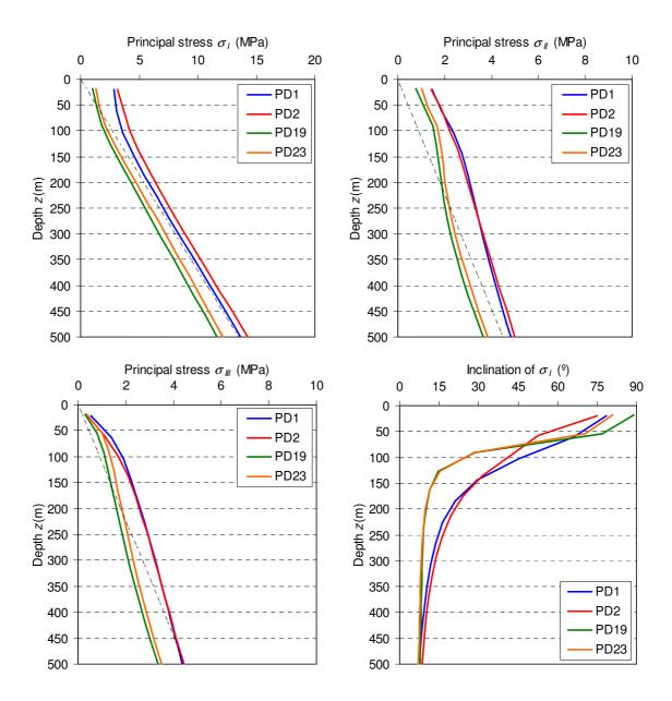
Figure 3.4: Variation with depth below the surface of the principal stresses ( $\sigma_l$ ,  $\sigma_{ll}$ ,  $\sigma_{ll}$ ) and the inclination of the maximum principal stress ( $\sigma_l$ ) with respect to the vertical direction.
