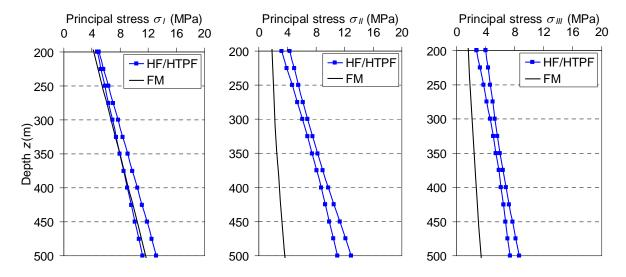
Figure 4: Variation of the magnitude of the principal stresses ( $\sigma_l$ ,  $\sigma_{ll}$ ,  $\sigma_{ll}$ ) obtained from the inversion of the hydraulic data (HF/HTPF) and with the FLAC3D model (FM) run with gravity loading only as functions of depth.
