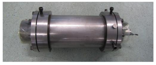
Figure 2.16: Biaxial test chamber with the core.
