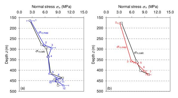
Figure 3.18: Variation with depth of the normal stress magnitudes as measured by hydraulic testing  $(\sigma_{n,mes})$  and computed with the FLAC3D model with  $\nu$ =0.47, considering gravity effects only, in boreholes (a) PD19 and (b) PD23.
