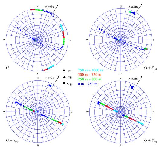
Figure 10. Orientation of the principal stresses obtained at the location of the borehole PD19 for the combined effect of gravity G and tectonic  $S_{yy}$  loadings.
