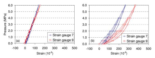
Figure 2.28: Pressure *versus* displacement curves obtained in biaxial tests performed in overcored cores. (a) linear and elastic behaviour; (b) non-linear and non-elastic behaviour.
