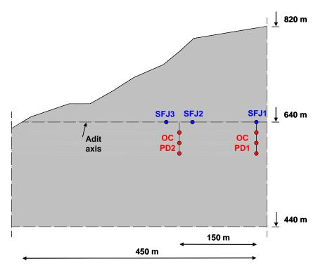
Figure 3: Vertical cutting plane along the adit axis showing the location of the overcoring and small flat jack tests.
