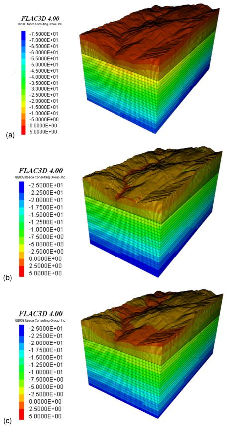
Figure 3.3: Contours of the principal stresses due to gravity loading: (a) maximum principal stress  $(\sigma_l)$ , (b) intermediate principal stress  $(\sigma_{ll})$ , and (c) minimum principal stress  $(\sigma_{ll})$ .
