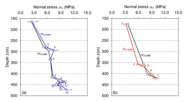
Figure 11: Variation with depth of the normal stress magnitudes as measured by hydraulic testing  $(\sigma_{n,mes})$  and computed with the FLAC3D model with  $\nu$ =0.47, considering gravity effects only, in boreholes (a) PD19 and (b) PD23.
