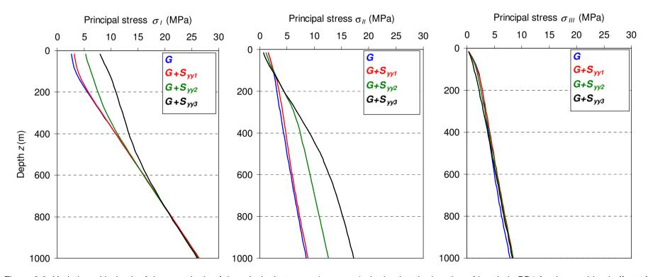
Figure 3.8: Variation with depth of the magnitude of the principal stresses ( $\sigma_l$ ,  $\sigma_{ll}$ ,  $\sigma_{ll}$ ) obtained at the location of borehole PD1 for the combined effect of gravity G and tectonic  $S_{yy}$  loadings.
