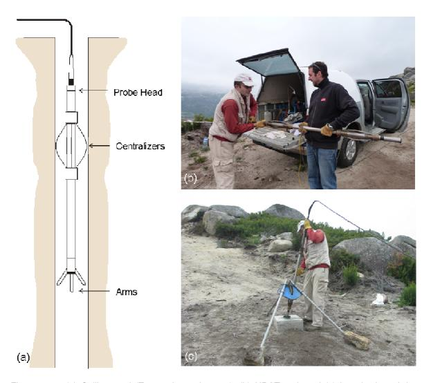
Figure 2.11: (a) Calliper tool (Zemanek *et al.*, 1969), (b) HRAT tool, and (c) introduction of the HRAT tool into borehole PD23.
