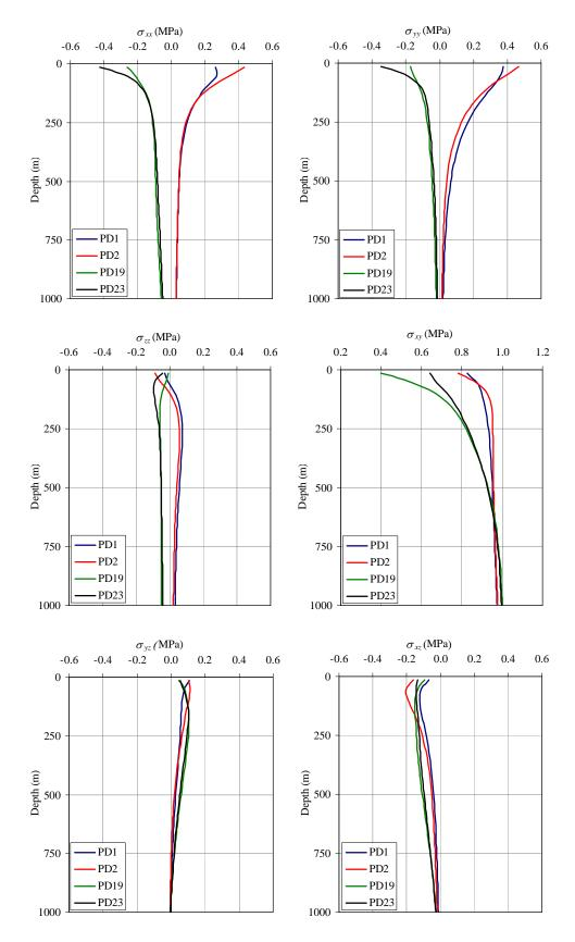
Figure 7. Variation of the stress tensor components for a unit shear stress  $S_{xy}$ .
