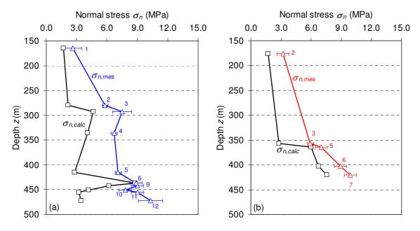
Figure 3.11: Variation of the magnitudes of the normal stresses obtained by hydraulic testing  $(\sigma_{n,mes})$  and with the FLAC3D model  $(\sigma_{n,calc})$  run with gravity loading only in boreholes (a) PD19 and (b) PD23 as a function of depth.
