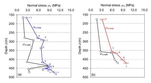
Figure 3: Variation of the magnitudes of the normal stresses obtained by hydraulic testing ( $\sigma_{n,mes}$ ) and with the FLAC3D model ( $\sigma_{n,calc}$ ) run with gravity loading only in boreholes (a) PD19 and (b) PD23 as a function of depth.
