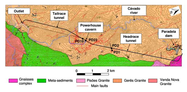
Figure 2.3: Layout of the Paradela II hydroelectric repowering scheme (courtesy of Energy of Portugal-EDP).
