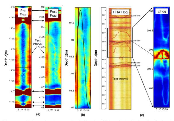
Figure 2.24: (a) Comparison between electrical imaging (EI) logs obtained before (Pre Frac) and after (Post Frac) a hydraulic fracturing test, (b) adjustment of the fracture plane with a sinusoidal curve and (c) identification of the main fracture planes in the electrical imaging (EI) and HRAT logs.
