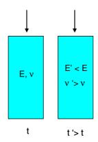
Figure 3.17: Soft linearly elastic material used for considering rheological effects.
