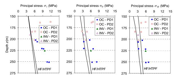
Figure 10: Comparison of the magnitudes of the principal stresses ( $\sigma_l$ ,  $\sigma_{ll}$ ,  $\sigma_{ll}$ ) obtained by overcoring and hydraulic testing.
