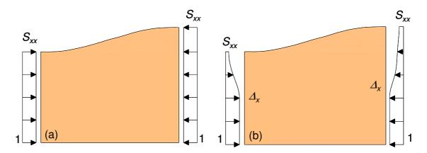
Figure 3.5: (a) Unbalanced stress state due to the effect of topography when a uniform stress  $S_{xx}$  distribution is applied at the boundaries of a numerical model (b) Uniform normal displacement  $\Delta_x$  applied at the boundaries to induce a horizontal unit stress  $\sigma_{xx}$  at the basal boundary of the model.
