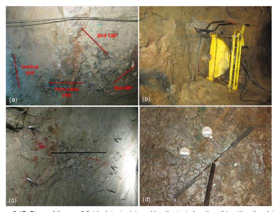
Figure 2.17: Steps of the small flat jack tests: (a) marking the tests location, (b) cutting the slot, (c) slot, anchor bolts and measurements pins, and (d) measuring the distance between the pins using digital transducers.
