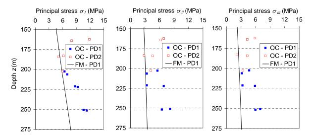
Figure 5: Variation of the principal stress magnitude ( $\sigma_l$ ,  $\sigma_{ll}$ ,  $\sigma_{ll}$ ) as obtained by overcoring (OC) and as computed with the FLAC3D model (FM) run with gravity loading only as functions of depth.
