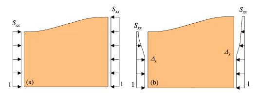
Figure 4. (a) Unbalanced stress state due to the effect of topography when a uniform stress  $S_{xx}$  distribution is applied at the boundaries of the numerical model (b) Uniform normal displacement  $\Delta_x$  applied at the boundaries to induce a horizontal unit stress  $\sigma_{xx}$  at the bottom boundary of the model.
