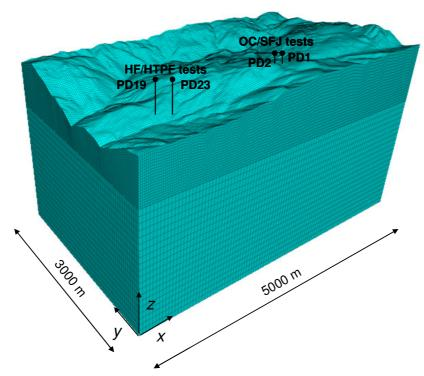
Figure 3.2: Mesh of the FLAC model.
