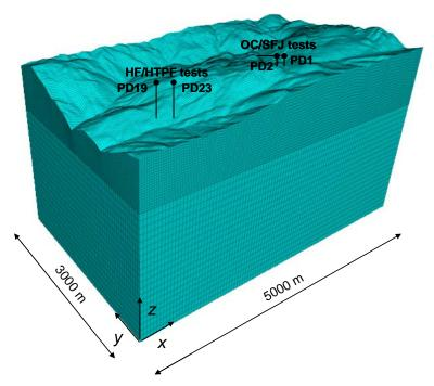
Figure 2: Mesh of the FLAC3D model.
