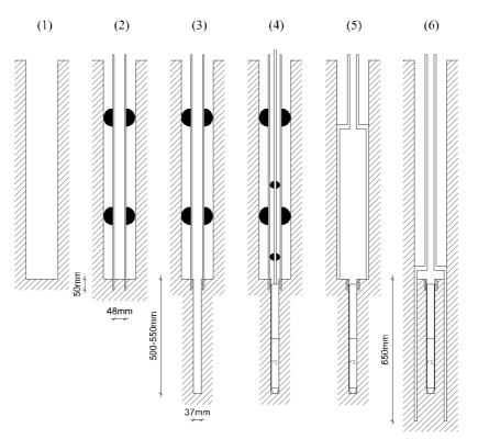
Figure 2.14: Sequence of execution of an STT stress measurement test.
