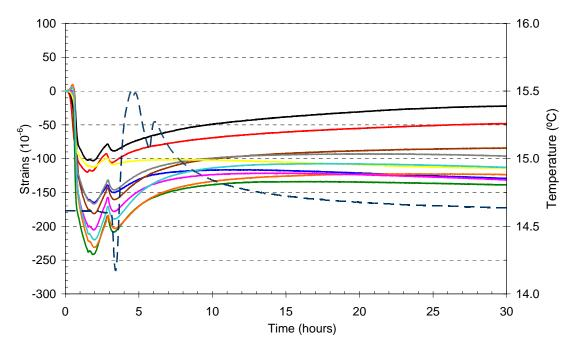
Figure 8: Strain versus time curves obtained during an overcoring test.
