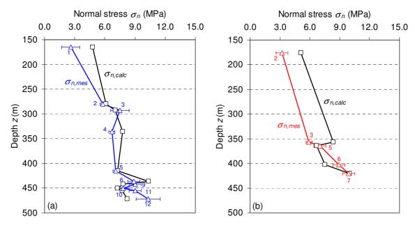
Figure 3.16: Variation with depth of the normal stress magnitudes as measured by hydraulic testing  $(\sigma_{n,mes})$  and computed with the FLAC3D model  $(\sigma_{n,calc})$  for the combined effect of gravity and tectonics in boreholes (a) PD19 and (b) PD23.
