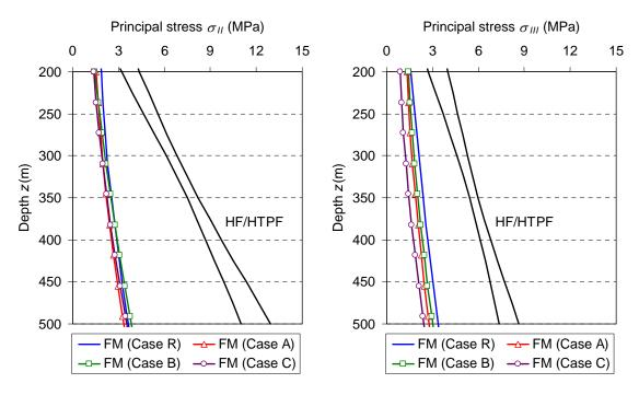
Figure 7: Variation with depth of the maximum ( $\sigma_{II}$ ) and minimum ( $\sigma_{III}$ ) sub-horizontal principal stresses obtained from the inversion of the hydraulic data (HF/HTPF) and with the FLAC3D model (FM) by considering the existing fractured zones.
