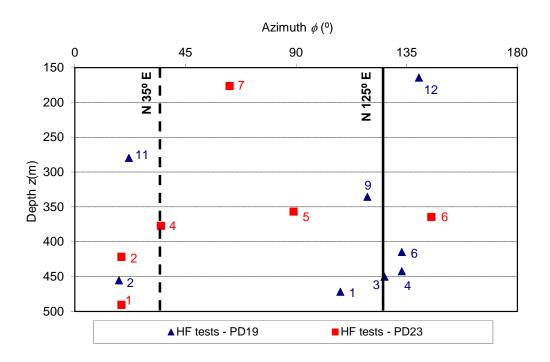
Figure 7: Variation of the azimuth  $\phi$  of the normal to the fracture planes obtained in hydraulic fracturing tests as a function of depth.
