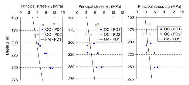
Figure 14: Variation with depth of the magnitude of the principal stresses ( $\sigma_l$ ,  $\sigma_{ll}$ ,  $\sigma_{ll}$ ) obtained by overcoring testing (OC) and with the FLAC3D model (FM) with  $\nu$ =0.47 considering gravity effects only.
