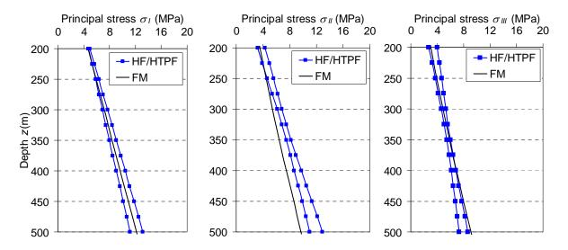
Figure 12: Variation with depth of the magnitude of the principal stresses ( $\sigma_l$ ,  $\sigma_{ll}$ ,  $\sigma_{ll}$ ) obtained from the inversion of the hydraulic data (HF/HTPF) and with the FLAC3D model (FM) with  $\nu$ =0.47 considering gravity effects only.
