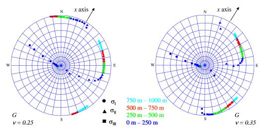
Figure 12. Orientations of the principal stresses obtained at the location of the borehole PD19 for the gravity loading with the values of 0.25 and 0.35 for the Poisson's ratio.
