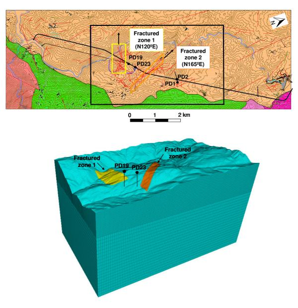
Figure 3.14: Location of the fractured zones in the FLAC3D model.
