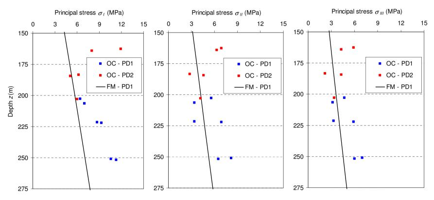
Figure 3.21: Variation with depth of the magnitude of the principal stresses ( $\sigma_l$ ,  $\sigma_{ll}$ ,  $\sigma_{ll}$ ) obtained by overcoring testing (OC) and with the FLAC3D model (FM) with  $\nu$ =0.47 considering gravity effects only.
