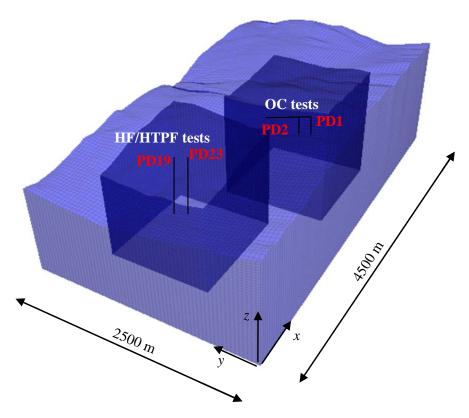
Figure 5. Three dimensional numerical model for Paradela site.
