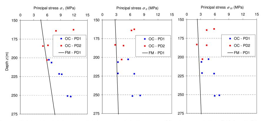
Figure 3.13: Variation of the principal stress magnitude ( $\sigma_l$ ,  $\sigma_{ll}$ ,  $\sigma_{ll}$ ) as obtained by overcoring (OC) and as computed with the FLAC3D model (FM) run with gravity loading only as functions of depth.
