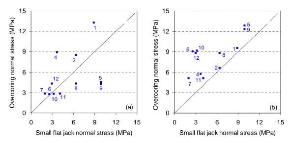
Figure 13: Comparison between small flat jack and overcoring normal stress considering the far-field stress tensor resulting from the (a) inversion of overcoring data and (b) shallow overcoring tests results.
