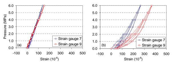
Figure 9: Pressure *versus* displacement curves obtained in biaxial tests performed in overcored cores. (a) linear and elastic behaviour; (b) non-linear and non-elastic behaviour.
