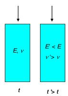
Figure 10: Soft linearly elastic material used for considering rheological effects.
