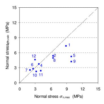
Figure 3.20: Comparison of the magnitudes of the normal stresses obtained by small flat jack technique ( $\sigma_{n,mes}$ ) and with the FLAC3D model ( $\sigma_{n,calc}$ ) with  $\nu$ =0.47 considering gravity effects only.
