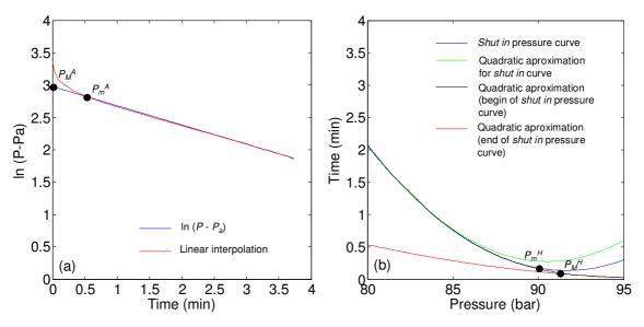
Figure 2.23: Determination of the shut-in pressure using the (a) Aamodt and Kuriyagawa's method and (b) Hayashi and Haimson's method.
