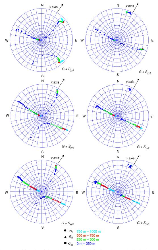
Figure 3.10: Orientation of the principal stresses obtained for the tectonic  $S_{yy}$  loading at the locations of boreholes PD1 (left) and PD19 (right).
