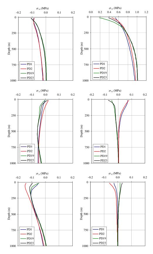
Figure 6. Variation of the stress tensor components for a unit tectonic stress  $S_{yy}$ .
