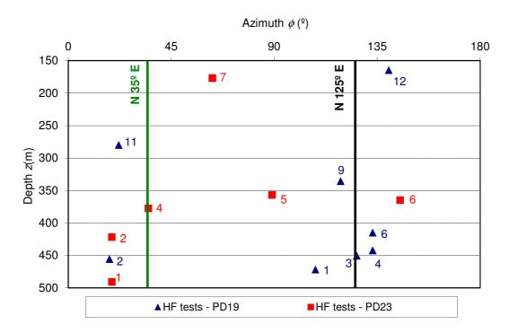
Figure 2.26: Variation of the azimuth  $\phi$  of the normal to the fracture planes obtained in hydraulic fracturing tests as a function of depth.
