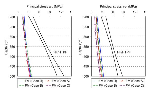
Figure 3.15: Variation with depth of the maximum ( $\sigma_{il}$ ) and minimum ( $\sigma_{il}$ ) sub-horizontal principal stresses obtained from the inversion of the hydraulic data (HF/HTPF) and with the FLAC3D model (FM) by considering the existing fractured zones.
