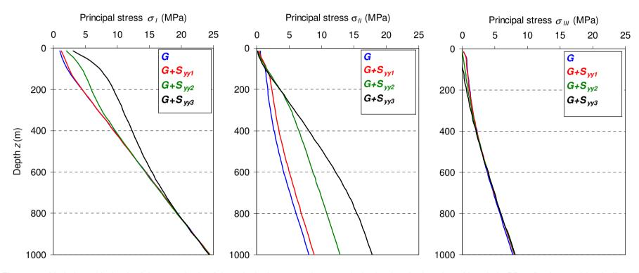
Figure 3.9: Variation with depth of the magnitude of the principal stresses ( $\sigma_{l}$ ,  $\sigma_{ll}$ ,  $\sigma_{ll}$ ) obtained at the location of borehole PD19 for the combined effect of gravity G and tectonic  $S_{yy}$  loadings.
