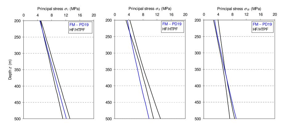
Figure 3.19: Variation with depth of the magnitude of the principal stresses ( $\sigma_l$ ,  $\sigma_{ll}$ ,  $\sigma_{ll}$ ) obtained from the inversion of the hydraulic data (HF/HTPF) and with the FLAC3D model with  $\nu$ =0.47 considering gravity effects only.
