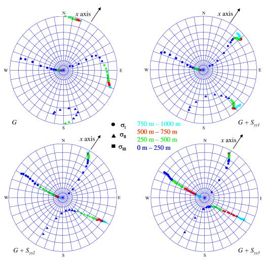
Figure 8. Orientation of the principal stresses obtained at the location of the borehole PD1 for the combined effect of gravity G and tectonic  $S_{yy}$  loadings.
