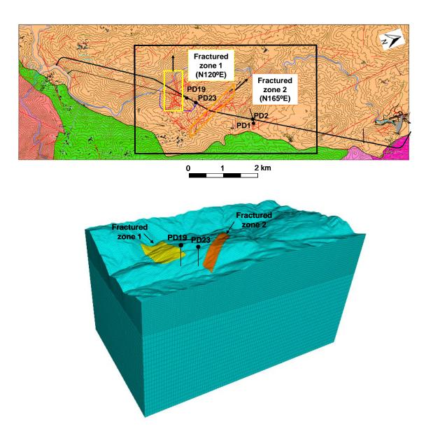
Figure 6: Location of the fractured zones in the FLAC3D model.
