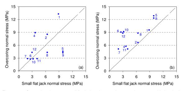
Figure 2.31: Comparison between small flat jack and overcoring normal stress considering the farfield stress tensor resulting from the (a) inversion of overcoring data and (b) shallow overcoring tests results.
