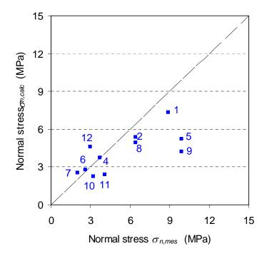
Figure 13: Comparison of the magnitudes of the normal stresses obtained by small flat jack technique  $(\sigma_{n,mes})$  and with the FLAC3D model  $(\sigma_{n,calc})$  with  $\nu$ =0.47 considering gravity effects only.
