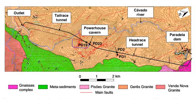
Figure 1: Layout of the Paradela II hydroelectric repowering scheme (courtesy of Energy of Portugal-EDP).
