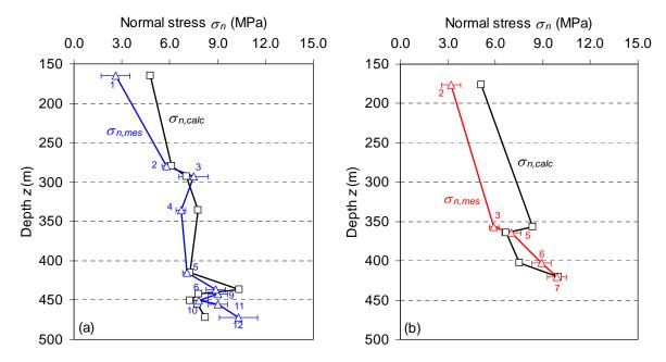
Figure 8: Variation with depth of the normal stress magnitudes as measured by hydraulic testing  $(\sigma_{n,mes})$  and computed with the FLAC3D model  $(\sigma_{n,calc})$  for the combined effect of gravity and tectonics in boreholes (a) PD19 and (b) PD23.
