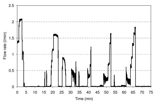
Figure 2.10: Record of test interval pressure and flow rate as a function of time through a hydraulic fracturing test.
