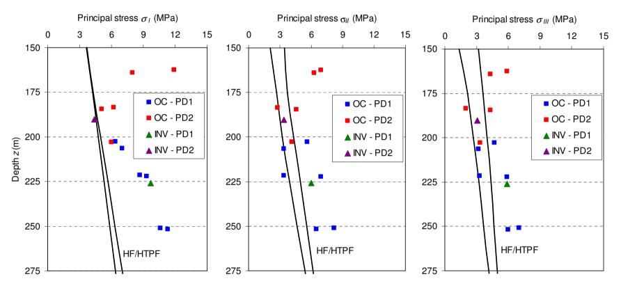
Figure 2.29: Comparison of the magnitudes of the principal stresses ( $\sigma_{l}$ ,  $\sigma_{ll}$ ,  $\sigma_{ll}$ ) obtained by overcoring and hydraulic testing.
