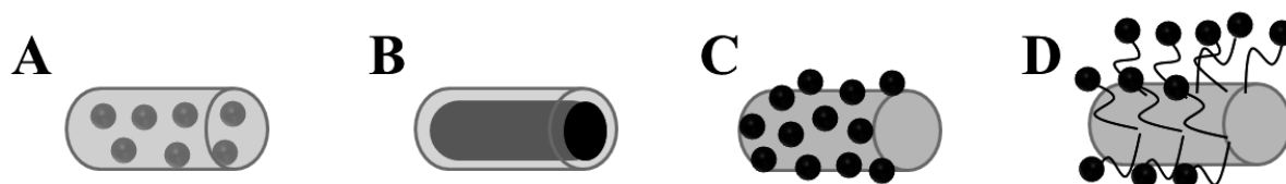
Scheme I.26. Several mechanisms of fiber functionalization: (A) blending of polymers prior electrospinning, (B) coaxial electrospinning, (C) physicochemical treatment and (D) surface immobilization
