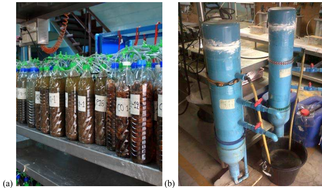
Figure 3.1. Reactors of the experiment (a) the reaction bottle for the batch experiment and (b) the column reactor for the continuous experiment.
