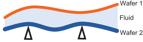
Fig. 22: Two wafers formulation. The top wafer is noted 1 and the bottom wafer, number 2.
