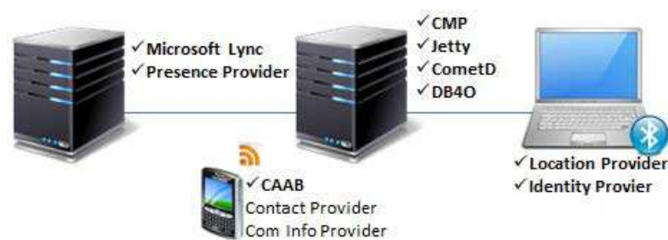
Figure 6.2: CAAB deployment architecture
