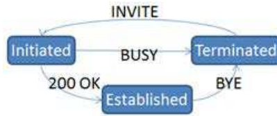
Figure 4.9: Call state transition in a SIP environment
