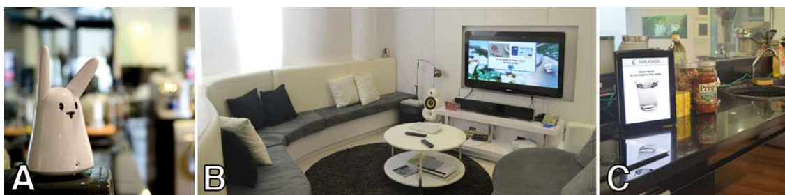
Figure 9.3: Photos of the Devices Deployed in STARhome A. Karotz, smart rabbit for sound, light and avatar movements in the bathroom B. IPTV with dedicated set-top box in the living room C. iPad with dedicated app in the kitchen
