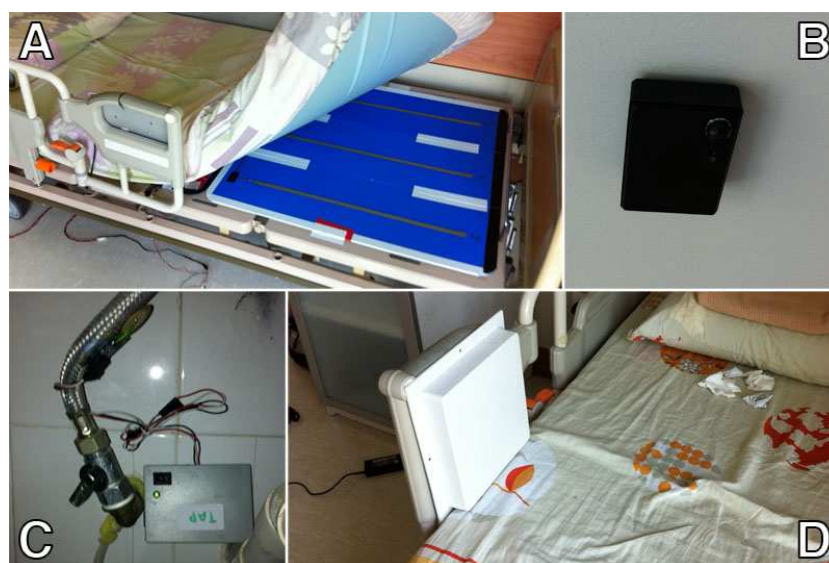
Figure 9.5: Photos of the Sensors Deployed in the Nursing Home
