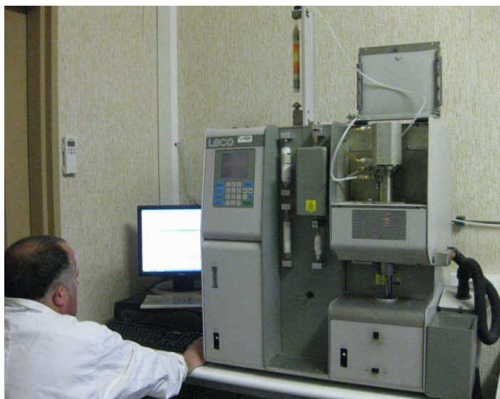
LECO CS 125 equipment
