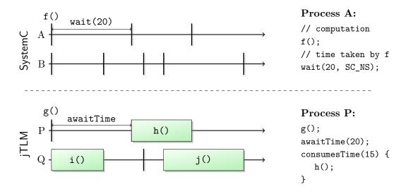
Figure 4.8: Time and Duration in SystemC and jTLM
