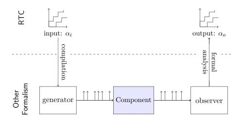
Figure 5.3: Connecting RTC to Other Formalisms
