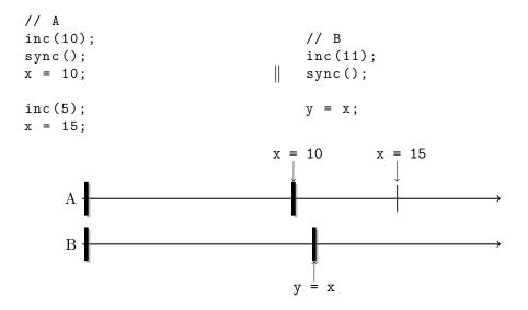
Figure 4.4: Example Reordering due to Temporal Decoupling
