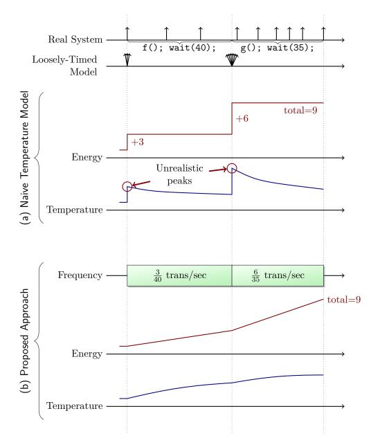
Figure 4.23: Elimination of Simulation Artifacts
