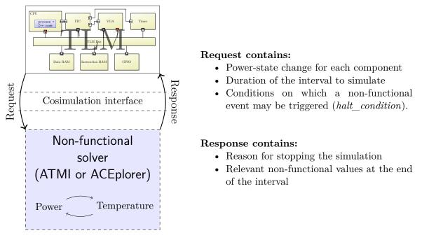
Figure 4.18: Cosimulation Interface
