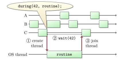
Figure 4.10: Execution of a during task (SystemC thread C calls during(42, routine))
