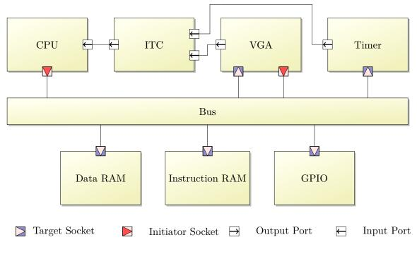
Figure 1.1: Graphical View of an Example TLM Platform
