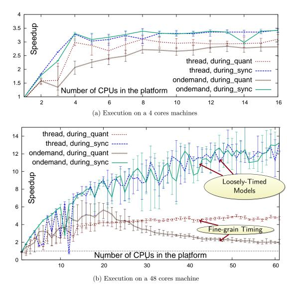
Figure 4.13: Speedup Compared to Sequential Simulation for Different Implementation (average, min and max over 10 runs)
