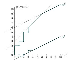
Figure 5.9: Example  $\mathcal{U}pac$  Curve:  $\alpha^u$  contains 3 explicit points and two affine pieces, and  $\alpha^l$  3 points and 1 affine piece
