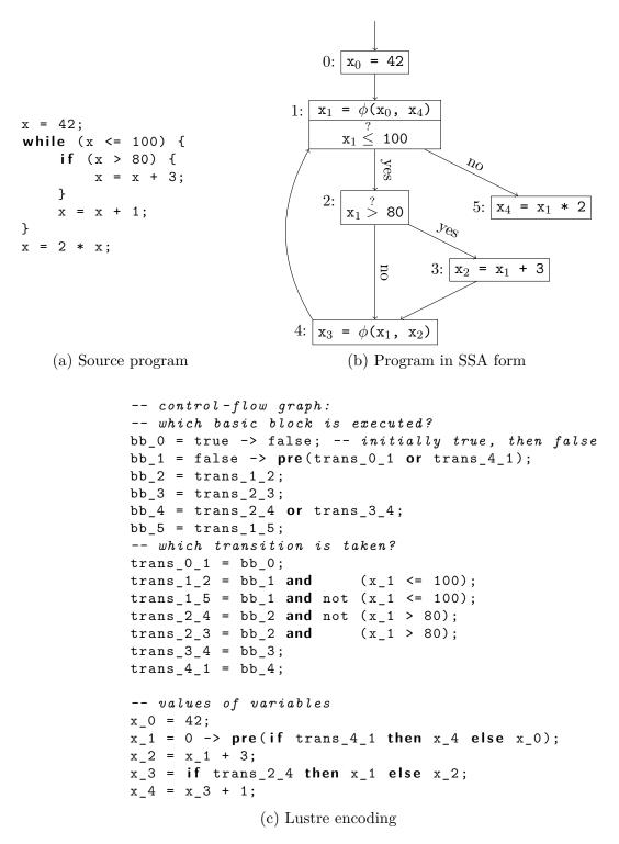
Figure 3.8: Imperative to synchronous, through SSA
