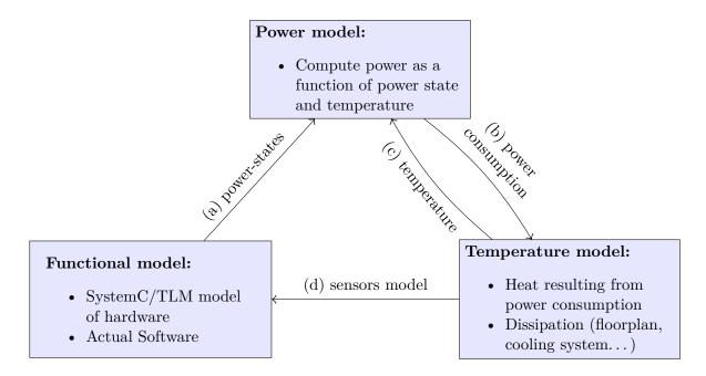
Figure 4.16: Functional, Power and Thermal Models
