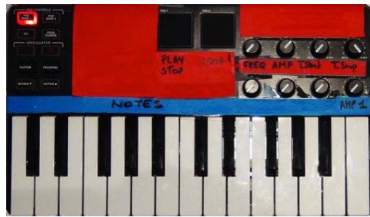
Figure 6.2: Figure 2: MIDI keyboard for playing with the harmonizer (in red) and the synthesizer (in blue).
