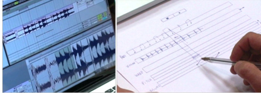
Figure 4.7: RD's prototype for sound editing. Left: Digital version of the recorded sound in Ableton Live software. Right: Paper interface with printed sequences of musical events (notes in a musical score and audio waveforms) aligned in time and horizontal zones for editing audio parameters (time stretching, pitch and amplitude) with the pen.
