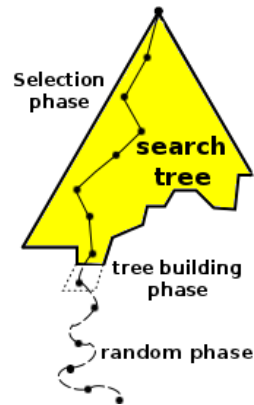
Figure 2.4: The search tree and three phases of the MCTS algorithm.
