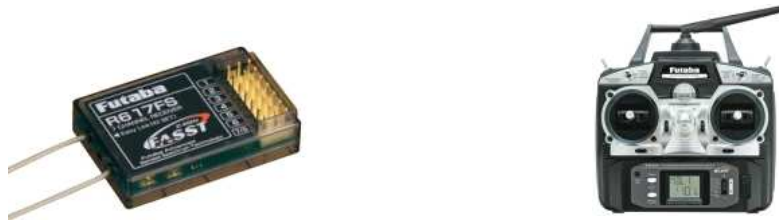
Figure 5-6: RC receiver Futaba R617FS and transmitter Futaba 6EX 2.4GHz.
