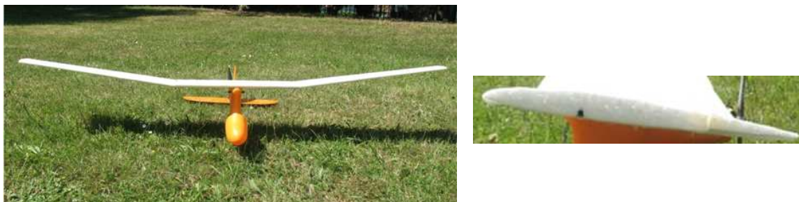
Figure 5-12: Illustration of the developed airfoil-shaped wing aircraft.
