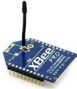
Figure 5-7: Xbee Pro 2.4 GHz.
