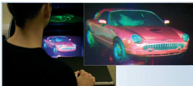
Figure 1.6: Replay of a spatial-multiplexed, 3 \times 8 billion-pixel, full-parallax, fullcolor, 3D image with a holographic display
