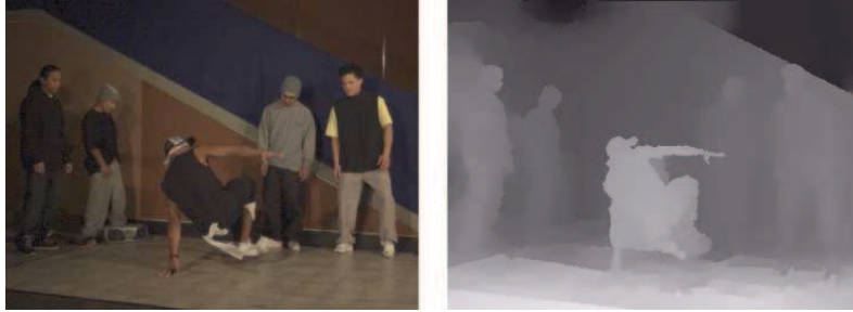
Figure 1.11: A texture frame and its associated depth map from the Breakdancers video sequence
