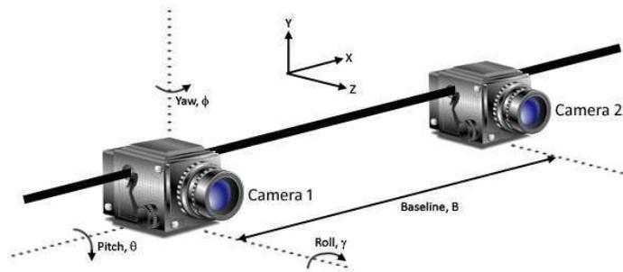
Figure 7.2: Depiction of the three axes of camera misalignment errors (the pitch, roll and yaw axis)[110].
