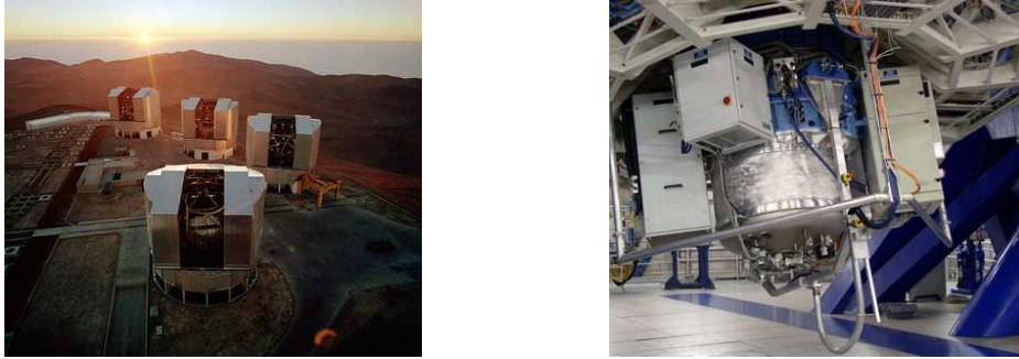
Figure 2.1: SINFONI (on the right) at VLT/UT4 (Yepen) Cassegrain focus (the foreground telescope on the photo of the left).
