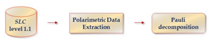
Figure 7.18 : First step of SAR processing chain: Pauli decomposition
