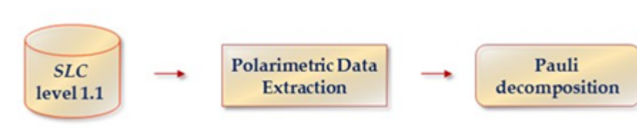
Figure 8.3 : First step of SAR processing chain: Pauli decomposition
