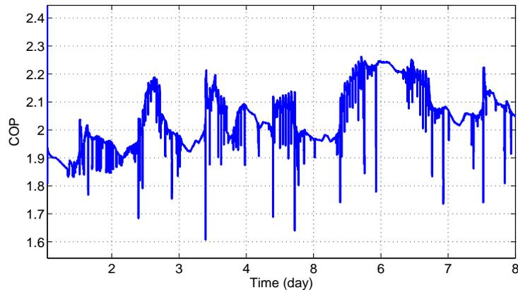
Figure 4.8: Winter heat pump energy efficiency factor (*COP*)
