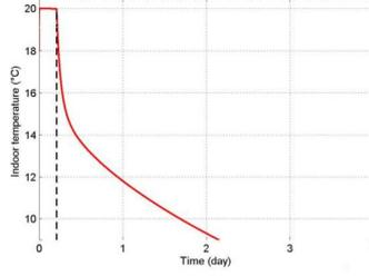
Figure 4.2: *All electrical house B* thermal step response
