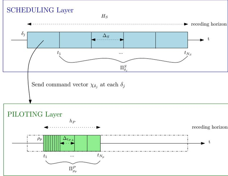
Figure 3.19: Principle of the Hierarchical Tracking mode
