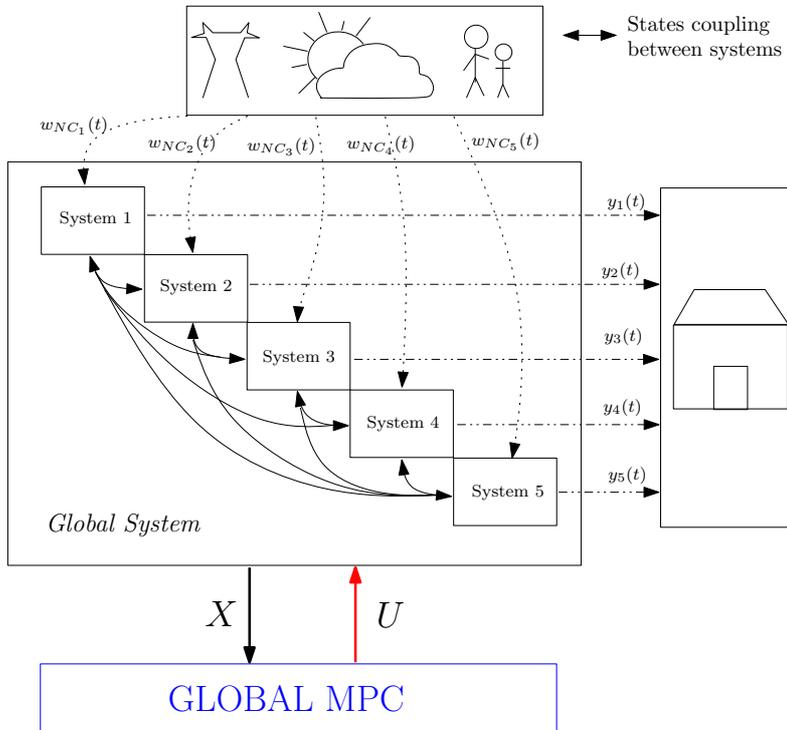
Figure 3.23: Diagram of the global BEMS with 5 systems
