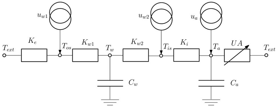
Figure 3.2: Electrical equivalent air thermal dynamic building model. The capacities  $C_w$  and  $C_a$  are associated to mass and air dynamics.  $R_i$  are the thermal resistances and  $u_i$  are the loads imposed on the different temperature nodes.
