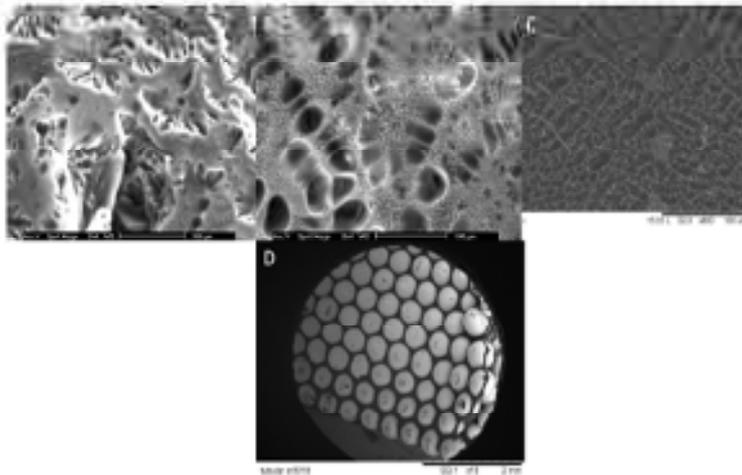
**Figure 1. Method of pore gradient formation.** Preparation of porous PLLA foams via freeze-extraction method. SEM micrographs (A) without macroporous titanium implants (outer); (B) with macroporous titanium implants (outer); (C) with macroporous titanium implants (inner). Presence of the implants changed the pore morphology. (C, D) Some process can be applied to tubular structures to obtain pore gradients in tubular implants. [Click here to view larger figure.](#)
