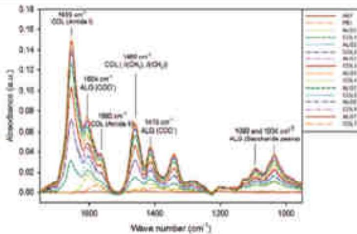
Figure 2. Evolution of FTIR-ATR spectra of a PEI/(ALG/COL) film during its buildup in 150 mM NaCl buffer solution (in D<sub>2</sub>O) at pH 3.8. Each spectrum was recorded after each deposition of a layer followed by the rinsing step.
