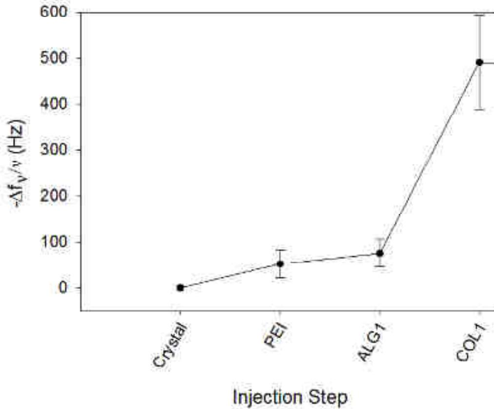
**Figure S1.** Buildup of PEI/(ALG/COL)<sub>7</sub> multilayer films on a SiO<sub>2</sub>-coated crystal followed by QCM-D. The buildup is performed at pH 3.8 (citrate buffer).
