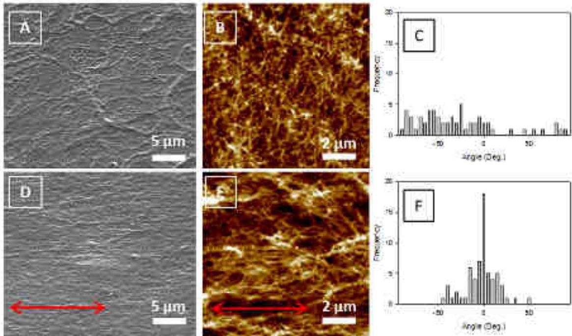
**Fig. 1.** Topography of collagen/alginate  $S_x$  films. SEM images of A)  $S_0$ , D)  $S_{100}$ . AFM images of B)  $S_0$ , E)  $S_{100}$ ; Distribution of the fibril angle for C)  $S_0$  and F)  $S_{100}$ . Fibril angles were obtained from images B) and E). Arrows show the direction of stretching and fibril alignment.
