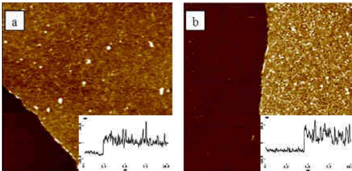
**Figure S5.** AFM observation of a PEI/(ALG/COL)<sub>3</sub> film cross-linked with (a) genipin at 100 mM, and (b) glutaraldehyde at 50 mM. The buildup was performed at pH 3.8. The cross-linking step was followed by a rinsing step at pH 7.4 after what they were brought back at pH 3.8 before imaging.
