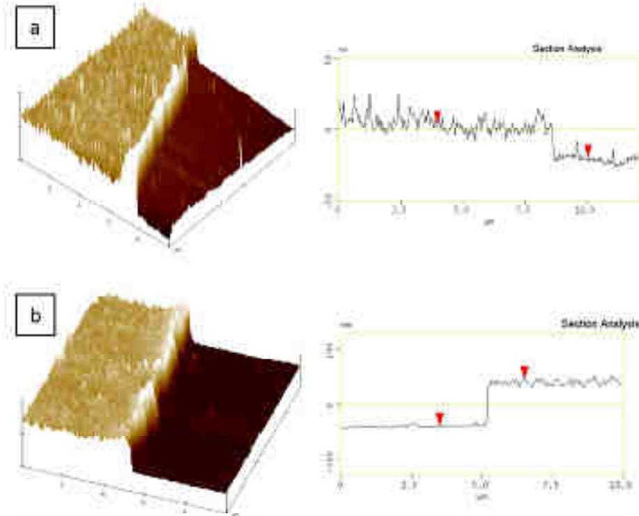
**Figure S2.** AFM observation of a (a) PEI/(ALG/COL)<sub>3</sub> film, and (b) a PEI/(ALG/COL)<sub>7</sub> film. The buildup was performed at pH 3.8. A scratch was performed to determine the thickness of the films. Image size is  $10 \times 10 \mu\text{m}^2$  and Z scale is 50 nm (a) and 100 nm (b).
