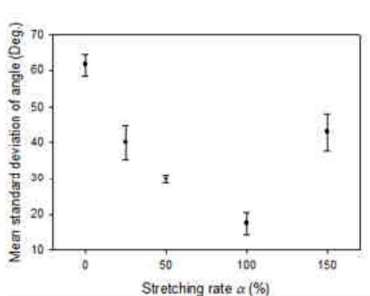
**Fig. 2.** Influence of the stretching rate on the alignment of collagen fibrils. Mean standard deviations were obtained from 6 images. Error bars correspond to the standard deviations of the 6 individual standard deviations taken from the 6 images.
