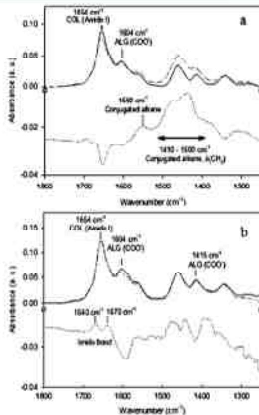
**Figure 8.** Evolution of the FTIR-ATR spectra of a PEI/(ALG/COL) film before (solid line) and after cross-linking (dashed line) with (a) genipin at 100 mM or (b) glutaraldehyde at 50 mM. Dotted lines difference between the two spectra. The film buildup step was performed at 150 mM NaCl in  $\text{D}_2\text{O}$  at pH 3.8. The cross-linking step was followed by a rinsing step at pH 7.4. Then the films were brought back to pH 3.8 before analysis.
