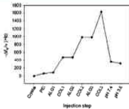
**Figure 5.** Buildup of a PEI/(ALG/COL)<sub>3</sub> multilayer film on a SiO<sub>2</sub>-coated crystal followed by QCM-D. Evolution of the opposite of the normalized frequency shift  $-\Delta f_i/v_i$  as a function of the injection step. The buildup is performed at pH 3.8 (citrate buffer) and at the end of the construction, the film is rinsed successively with a HEPES buffer at pH 7.4 and a citrate buffer at pH 3.8.
