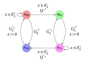
Figure 2.10: Parametric timed automaton modeling a "NOT" gate
