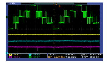
Figure 9.12: Output voltage (above) and capacitor voltages (below) in presence of time-varying period *T*
