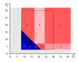
Figure 2.13: Behavioral cartography of the flip-flop according to  $\delta_3^+$  and  $\delta_4^+$
