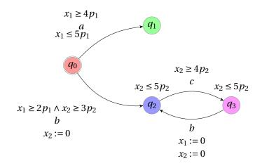
Figure 2.4: An example of a parametric timed automaton
