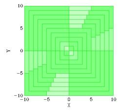
Figure 8.23: Nested decompositions for boost DC-DC converter found by starting from  $R = [0, 10] \times [0, 4]$
