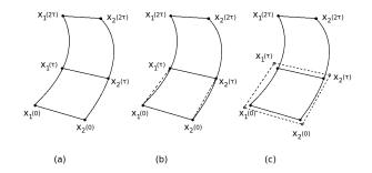
Figure 7.7: (a) A segment  $F = [x_1(0), x_2(0)]$  and its exact segment successor  $[x_1(\tau), x_2(\tau)]$  at time  $\tau$ . (b) Approximating the set of continuous trajectories starting from F during  $\tau$  time by convex hull (c) Bloating the convex polyhedron to obtain a polyhedral over-approximation (from [ABD<sup>+</sup>00])
