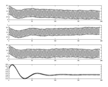
Figure 7.18: Discrete-time trajectory of 3-cells converter starting at  $x_0 = (5,5,5,16)$  in  $S = [4,7] \times [4,7] \times [4,7] \times [15,17]$  using the direct control method (from top to bottom:  $x_1, x_2, x_3, x_4$  in function of time)
