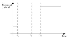
Figure 7.3: Staircase command signal u(t) issued by the actuator as it receives controller symbols  $\tilde{u}[1], \tilde{u}[2], \ldots$  at time  $t_1, t_2, \ldots$  (from [AK02])
