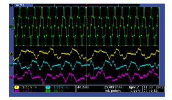
Figure 9.10: Zoom of output voltage (above) and capacitors voltages (below)
