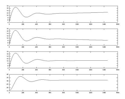
Figure 7.20: Trajectory of the 3-cells converter starting at  $x_0 = (5.4, 5.4, 5.4, 16)$  with switching rule  $(4 \cdot 4 \cdot 4 \cdot 1 \cdot 21)^*$  found by the indirect method (precision  $\varepsilon = 21.6$ )
