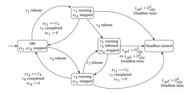
Figure 4.2: PSA modelling a preemptive processor with two tasks  $\tau_1, \tau_4$
