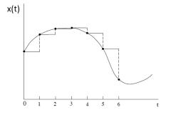
Figure 7.4: Controller symbols  $\tilde{x}[1], \tilde{x}[2], \dots$  produced by the generator by sampling of the plant output signal x(t) (time-triggered plant event model) (from [AK02])
