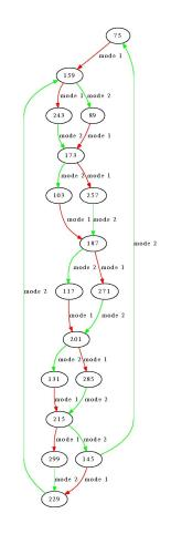
Figure 7.13: Graph of an abstract safety controller of the boost DC-DC converter, with  $\eta = \frac{1}{40}$  and  $S = [3, 3.4] \times [1.5, 1.8]$  obtained by a script of ours
