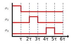
Figure 7.17: Switching rule for the 3-cells boost DC-DC converter on one period of length  $6\tau$ ,  $\sigma_1 = (1 \cdot 0^5)$ ,  $\sigma_2 = (0^2 \cdot 1 \cdot 0^3)$ ,  $\sigma_3 = (0^4 \cdot 1 \cdot 0)$ , and the corresponding control pattern is  $(2 \cdot 1 \cdot 3 \cdot 1 \cdot 5 \cdot 1))$
