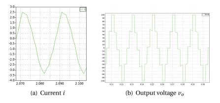
Figure 9.5: Current and output voltage
