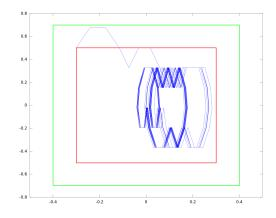
Figure 8.10: Unfolded  $\Delta$ -trajectory of helicopter motion in plane  $(x, \dot{x})$  starting at (-0.3, 0.5) (inner box: *R*, outer box: *S*)
