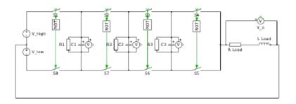
Figure 9.2: Electrical scheme of a 5-level converter
