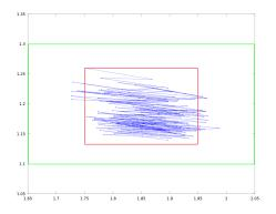
Figure 8.30: Unfolded  $\Delta$ -trajectory of the boost converter with disturbances in plane ( $i_l$ ,  $v_c$ ), starting at (1.75, 1.26) (inner box:  $R = [1.75, 1.95] \times [1.14, 1.26]$ , outer box:  $S' = [1.65, 2.05] \times [1.1, 1.3]$ )
