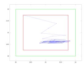
Figure 8.13: Unfolded  $\Delta$ -trajectory of heating system in plane ( $T_1$ ,  $T_2$ ), starting at (20.25, 21.75) (inner box  $R = [20.25, 21.75] \times [20.25, 21.75]$ , outer box  $S = [20, 22] \times [20, 22]$ )
