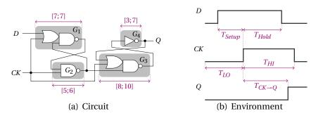
Figure 2.9: Flip-flop circuit and its environment
