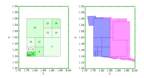
Figure 8.6: Left: decomposition  $\Delta$  for boost converter of  $R = [1.75, 1.95] \times [1.14, 1.26]$ ; right:  $\Delta$ -unfolding where dark gray (resp. light gray) indicates mode 1 (resp. 2), with enclosing box  $S = [1.7, 2.0] \times [1.1, 1.3]$
