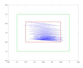
Figure 8.7: Unfolded  $\Delta$ -trajectory of the boost converter starting at (1.75, 1.26) (inner box  $R = [1.75, 1.95] \times [1.14, 1.26]$ , outer box  $S = [1.7, 2.0] \times [1.1, 1.3]$ )
