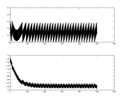
Figure 7.11: Discrete-time trajectory starting from point  $x_0 = (3.01, 1.79)$ , using the control found by the direct method. Above: evolution of  $v_c$  in time; below: evolution of  $i_l$ .
