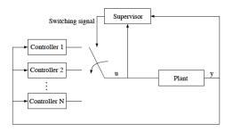
Figure 7.5: Scheme of a switching controller feedback controller
