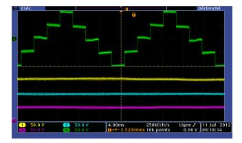
Figure 9.9: Output voltage and capacitor voltages
