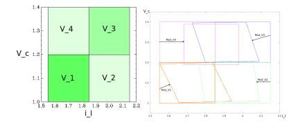
Figure 8.1: Decomposition  $\Delta$  of  $R = [1.55, 2.15] \times [1.0, 1.4]$  for the Boost DC-DC converter example (left), and visualization of  $Post_{\Delta}(V_i) \subset R$ , i = 1, ..., 4 (right)
