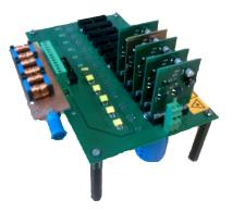
Figure 7.15: 3-cells converter built by SATIE Electronics Laboratory
