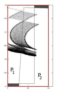
Figure 7.10: Maximal controlled invariant subset of  $S = [3.0, 3.4] \times [1.5, 1.8]$ , composed of two polyhedra  $P_1$  (mode 1) and  $P_2$  (mode 2), with a controlled trajectory starting at  $x_0 = (3.01, 1.79)$
