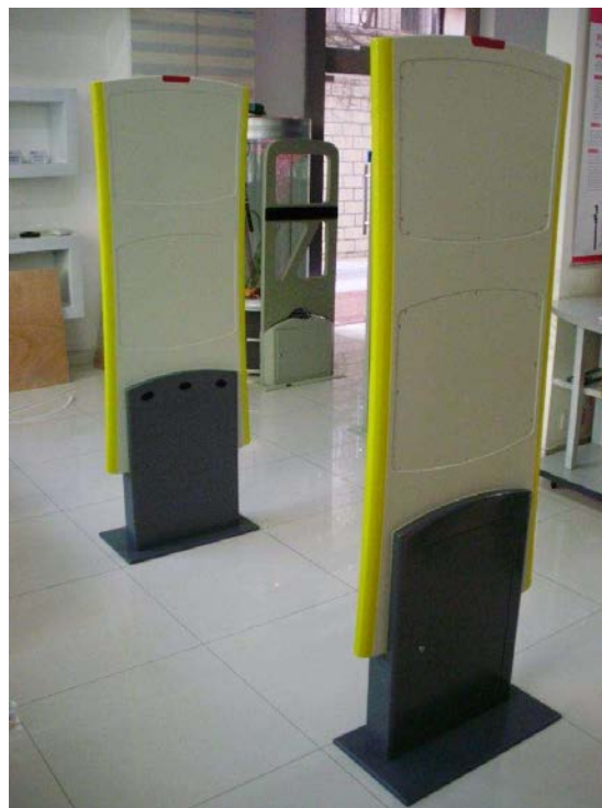
Figure 1.12: Using two RFID readers for “spatial” coverage
