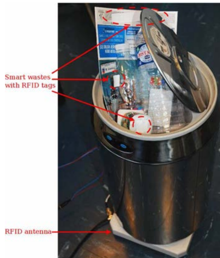
Figure 3.3: A collective bin using the RFID technology.
