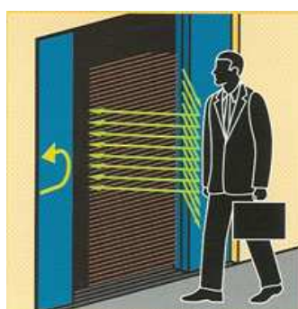
Figure 1.8: Automatic doors using Infrared
