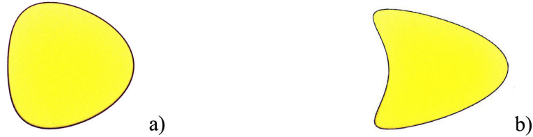
Figure 6.20: Disk contour deformation into a kite: a) convex shape with \delta = 0.165 , b) concave shape with \delta = 0.5 .
