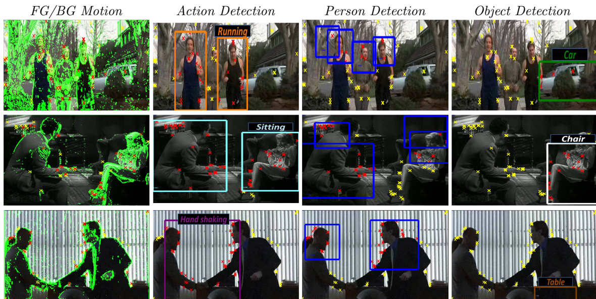
Figure 4.5: Illustration of proposed semantic region extraction in video according to (from left to right): motion region segmentation, action detection, person detection and object detection. Correct segmentation separates local features into meaningful groups denoted by yellow and red crosses. We also illustrate failures of automatic segmentation due to false negative detections (see e.g., missed running action in the first row) and false positive detections (see e.g., incorrect table detection in the third row ).
