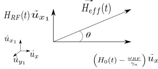
Figure B.2: Magnetic fields scheme in the neutron rest frame rotating at the frequency  $\omega_{\text{RF}}$  around the  $\vec{H}_0$  axis.
