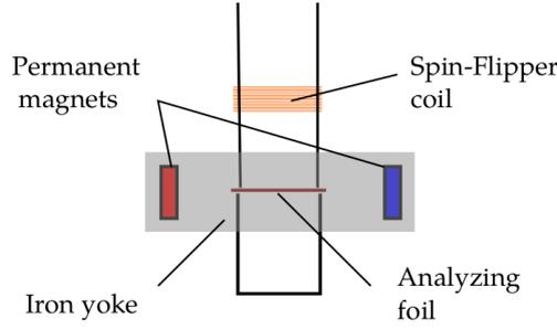
Figure 3.12: Scheme of the spin analysing system.
