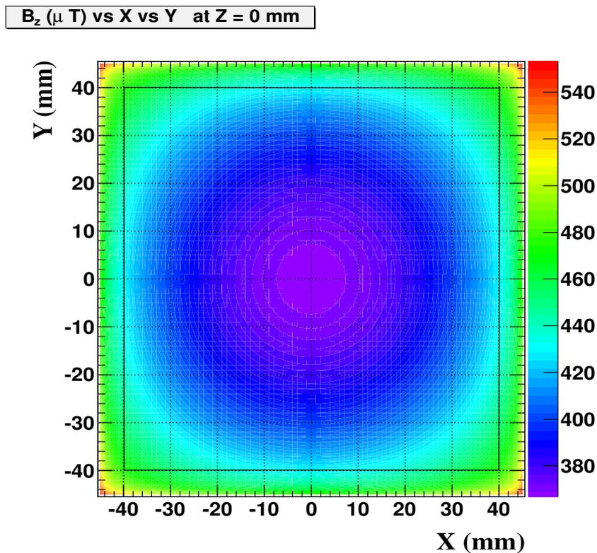
Figure 5.4: Cross view of the RF magnetic field amplitude produced by 1 A at the centre of the spin-flipper from Maentouch [91]. Limits of the UCN guide are shown by the full black line.
