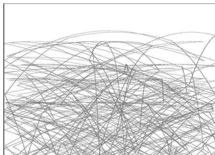
Figure 2.11: Parabolic UCN trajectories simulated using GEANT4-UCN, as an example of the gravity effect on ultra cold neutrons.
