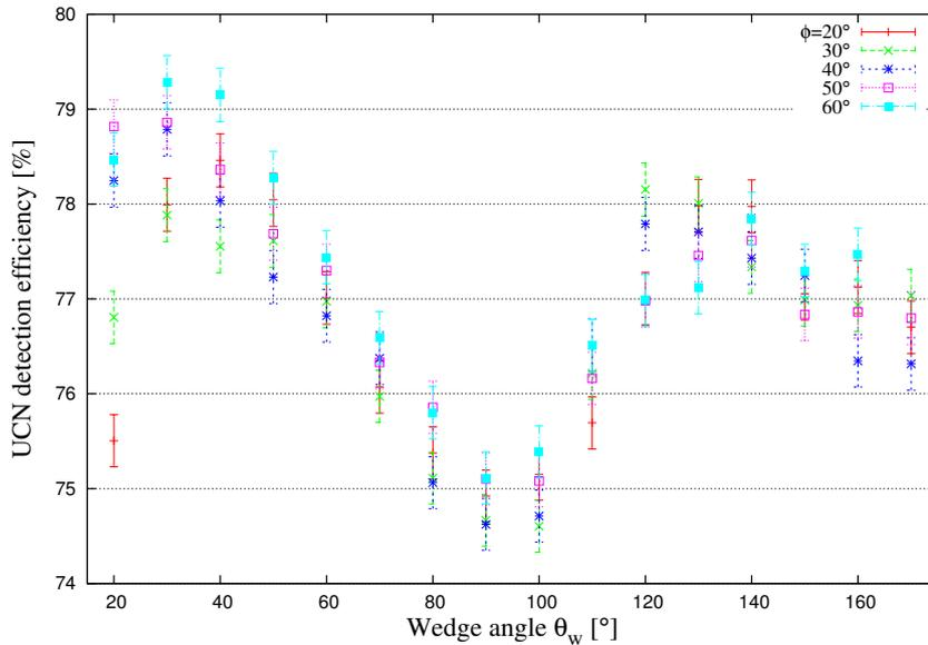
Figure 4.10: USSA detection efficiency as a function of the  $\theta_w$  wedge angle for different values of the roof angle  $\phi$ . No influence of the roof angle on the USSA detection efficiency is observed. The best wedge angles are around 30 and 130°.
