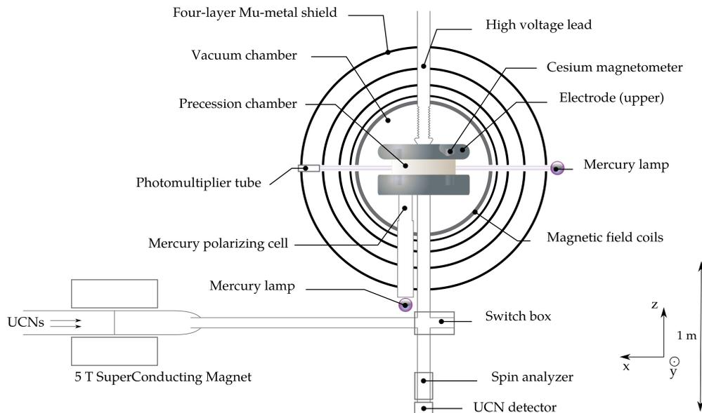
Figure 3.3: Sketch of the nEDM apparatus. The big surrounding field compensation coils (SFC) are not shown. On the bottom right corner of this figure, the nEDM reference frame axes used throughout this work is defined. It is centred on the Hg readout level at the centre of the precession chamber.
