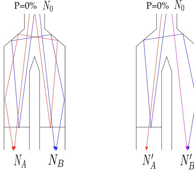
Figure 5.20: USSA configurations used to determine the reflection probability from the wrong spin detection arm to the right one. In one case, the two analysing foils are installed. In the other case, one foil is removed.
