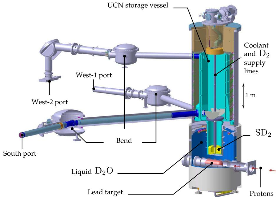
Figure 3.2: Sketch of the PSI ultra cold neutron source with its three available beam ports. The nEDM experiment is connected to the South beam port.
