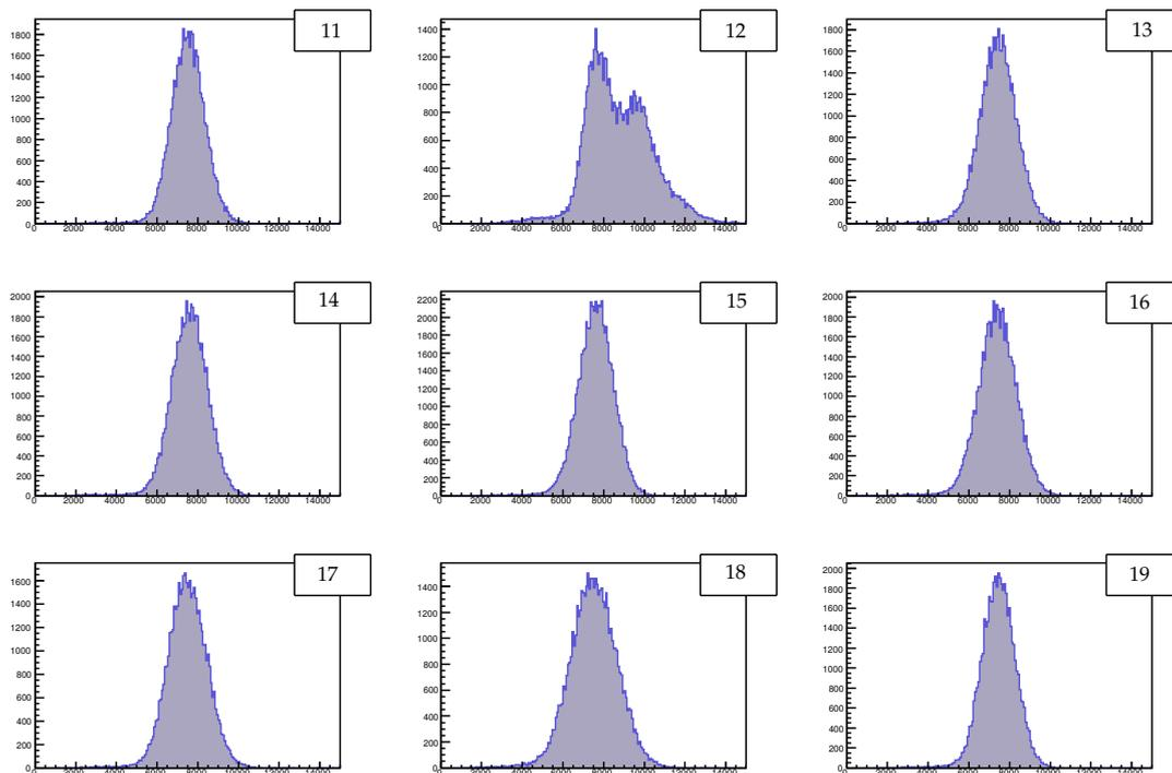
Figure 5.2: Charge distribution measured with NANOSC B at PSI in August 2013 over one cycle (threshold: 3 mV, validation gate: 12 ns). The  $y$  axis is the number of count for a given QDC value (arbitrary unit). The shoulder on the UCN peak of channel 12 might be due to a bad optical contact between the pipe guide and the photomultiplier or to the PMT. The whole channel (PMT, light pipe and scintillators) has been exchanged for 2014.
