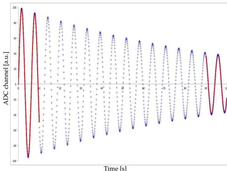
Figure 6.5: Illustration of the two windows method used by the RAL-Sussex-ILL collaboration to extract the Hg Larmor precession frequency.
