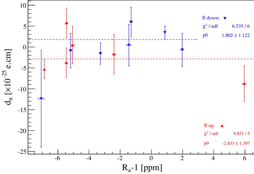
Figure 6.17: Constant fits of the  $B_0$  up and the  $B_0$  down nEDM data.  $B_0$  up correspond to the up red triangles and  $B_0$  down to the down blue triangles.
