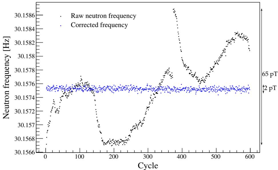
Figure 6.6: Illustration of the correction of magnetic field drifts using the Hg normalisation on the neutron resonant frequency over a 60 h long run. Error bars, of the order of 22  $\mu$ Hz ( $\sim 800$  fT) for this data set, are omitted for clarity.
