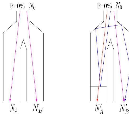
Figure 5.15: USSA configurations used to determine the reflection probability from the wrong spin detection arm to the good one on the West-2 beam line. In one case there is no foil. In the other case, a single analysing foil is added.
