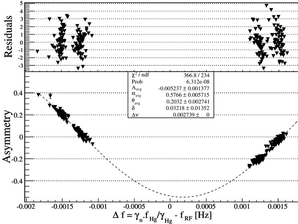
Figure 6.3: Asymmetry fitting procedure used to extract the neutron Larmor frequency. In order to compensate for magnetic field variations, the  $\pi/2$  pulse frequency is normalised by the mercury frequency.
