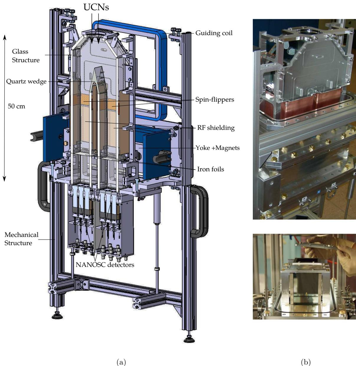
Figure 5.1: Left panel: Cut view of USSA mechanical drawing. Upper right panel: open view of the USSA with visible RF shielding and vacuum chamber. Lower right panel: installation of USSA analysing foils.
