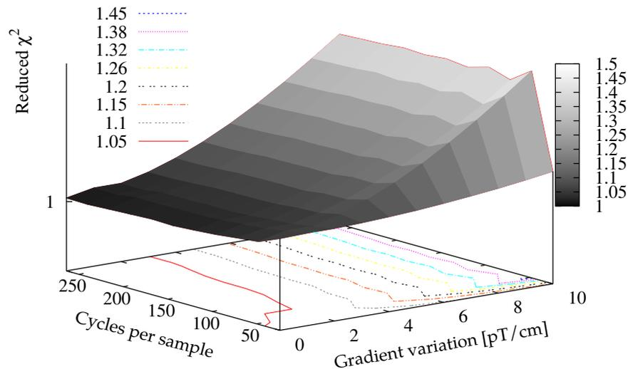
Figure 6.15: Map of the reduced  $\chi^2$  as a function of the number of cycles used to perform the fit and the amplitude of the daily gradient variation. Toy data have been produced using a 50 pT/cm static gradient.
