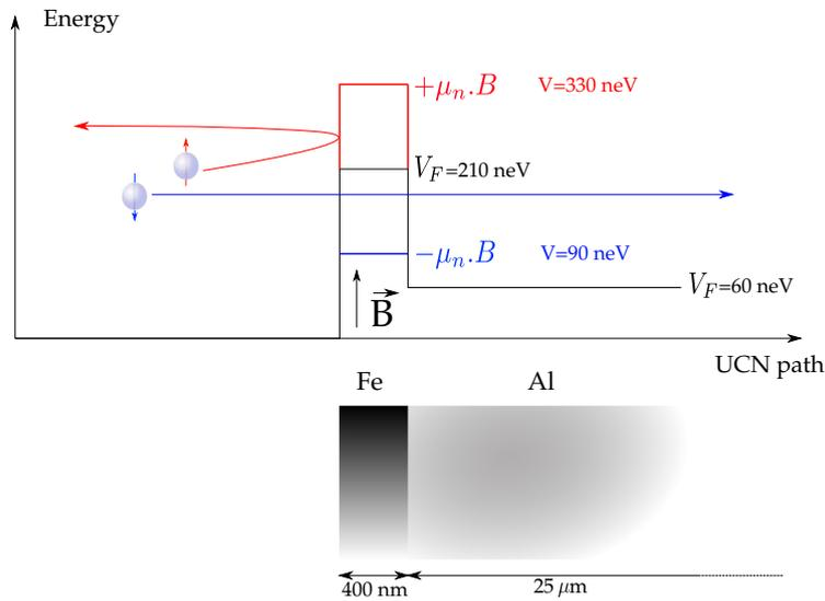
Figure 3.13: Sketch of the spin analyser principle.
