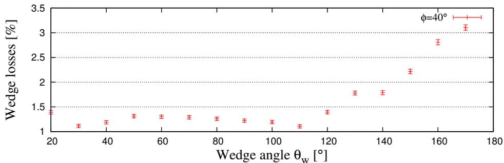
Figure 4.12: Central wedge losses as a function of the wedge angle  $\theta_w$  for  $\phi = 40^\circ$ .
