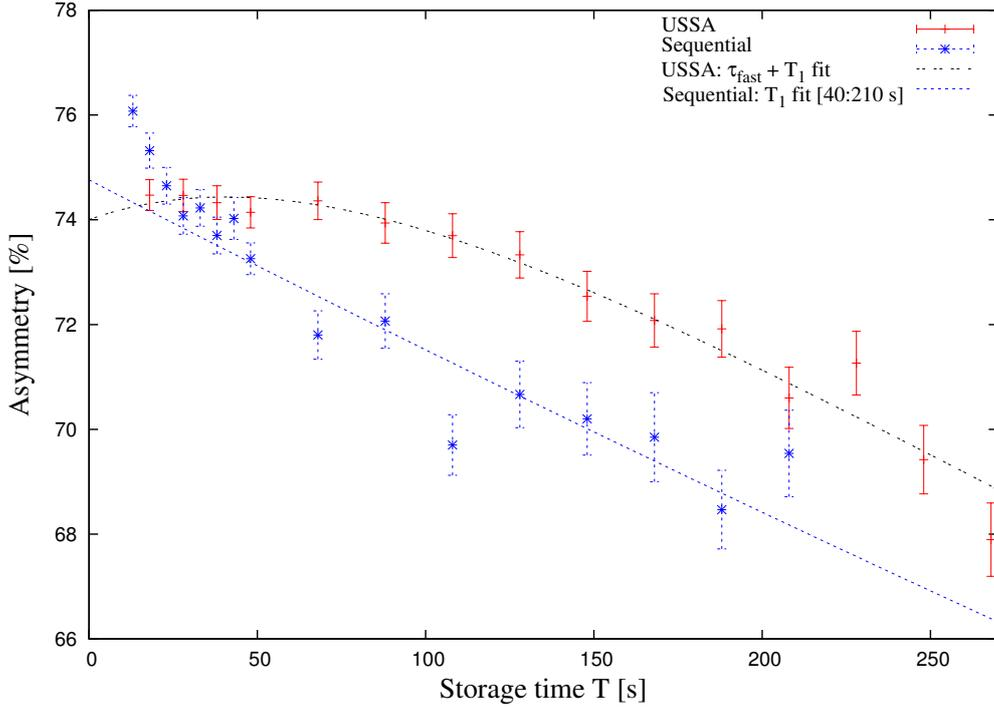
Figure 5.18: Asymmetry as a function of storage time for the USSA (red cross) and the sequential system (blue star) during  $T_1$  measurement. The black dashed line corresponds to the USSA data fit using Eq (5.19). The blue dash line corresponds to the usual  $T_1$  fit applied to the sequential analyser data between 40 and 210 s.
