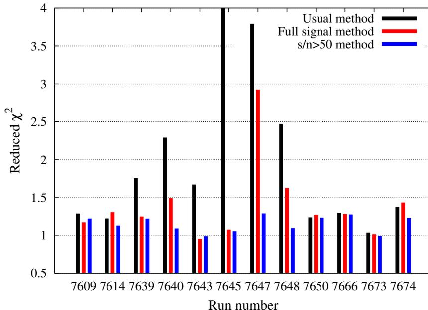
Figure 6.7: Reduced  $\chi^2$  of the neutron Larmor frequency fit averaged over all electric field polarities using different Hg frequencies (according to the method used to extract the Hg frequency). Here, the usual method is the method used by the RAL-Sussex-ILL collaboration to extract the Hg frequency. The  $\tilde{\chi}^2$  for the run 7645 with the usual method of about 10 is not shown in this figure.
