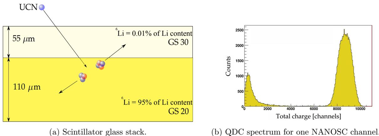
Figure 3.11: Stack principle and obtained charge spectrum for one NANOSC channel.
