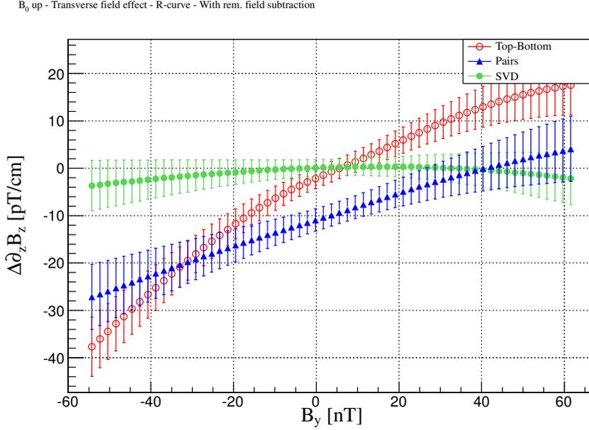
Figure 7.5: Difference between the estimated gradients and the reconstructed map gradient as a function of the  $B_y$  field component strength. The field is only reconstructed using the  $B_0$  coil (up direction) and the H1B coil.
