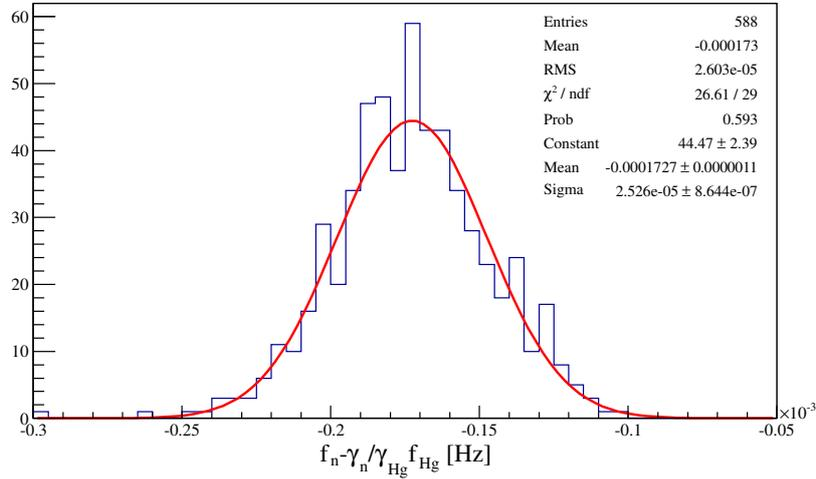
Figure 6.9:  $f_n - \frac{\gamma_n}{\gamma_{\text{Hg}}} f_{\text{Hg}}$  distribution obtained in the run 7650. It is not centred on 0 because of the gravitational shift due to a magnetic field gradient (measured to about 27 pT/cm with CsM).
