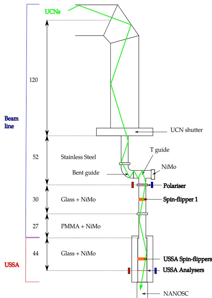
Figure 5.11: West-2 beam line setup.
