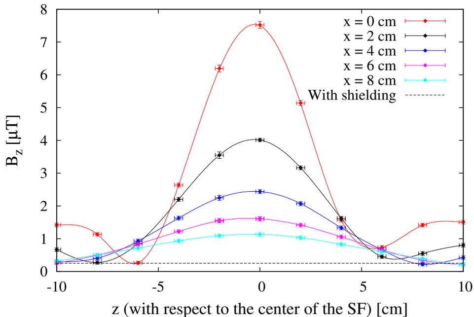
Figure 5.6:  $B_z$  amplitude along  $z$  in different  $x$  planes in the non-active spin-flipper without shielding for diamond points. Lines are just used to guide eyes. The black dash line corresponds to the highest measured amplitude with the RF shielding.
