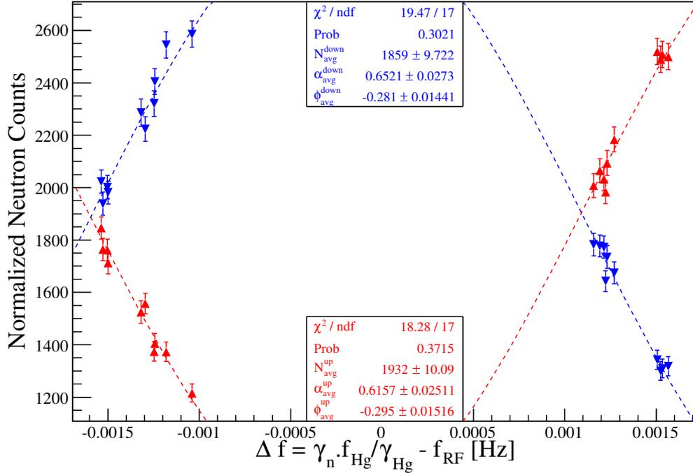
Figure 5.21: First Ramsey pattern taken with the USSA (in  $B_0$  up configuration).
