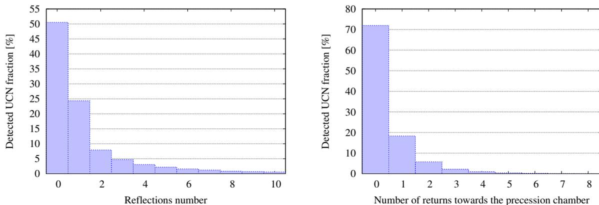
(a) Reflections number per UCN on the foil located in the wrong analysing arm. (b) Number of returns towards the precession chamber.
