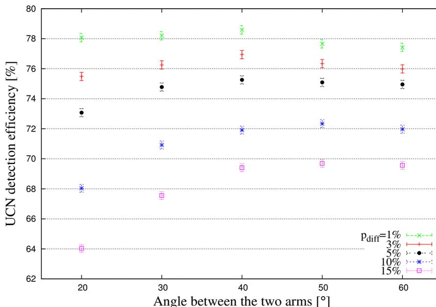
Figure 4.6: YSSA UCN detection efficiency as a function of the  $\theta$  angle between the two analysing arms. The simulation has been performed for several diffuse probabilities  $p_{\text{diff}}$  in the two arms.
