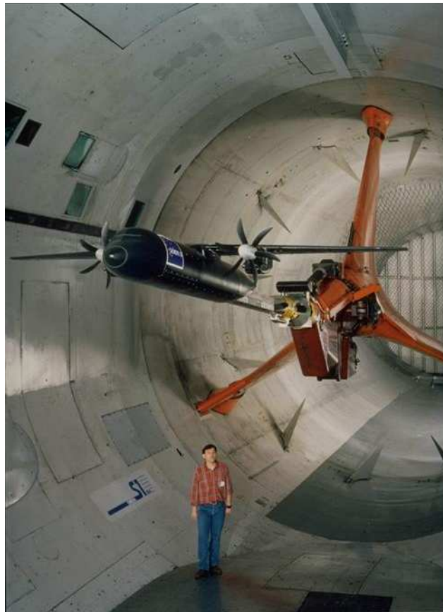
Figure 4: Gemini II full-aircraft model at Onera S1MA transonic wind tunnel facility
