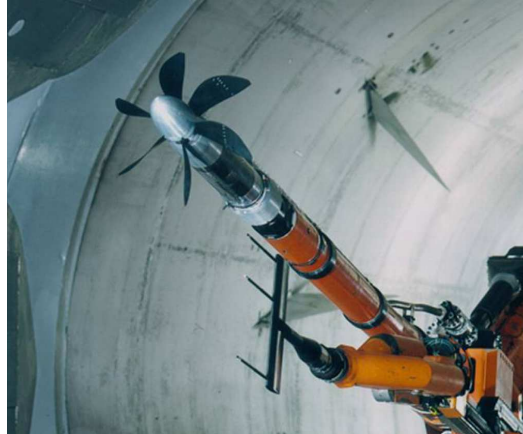
Figure 31: APIAN propeller minimum-body configuration in Onera-S1MA wind tunnel facility
