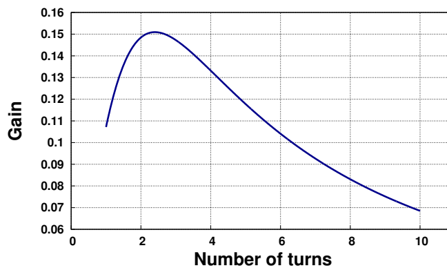
Figure 4.22: Simulation of the gain of a tuned flux transformer at \omega_0 according to the number of pickup coil's turn
