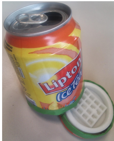
Figure 5.9: Teflon phantom in an aluminum can.
