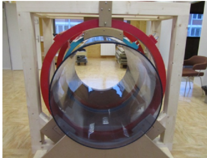
Full-head setup for MRI at very low field
