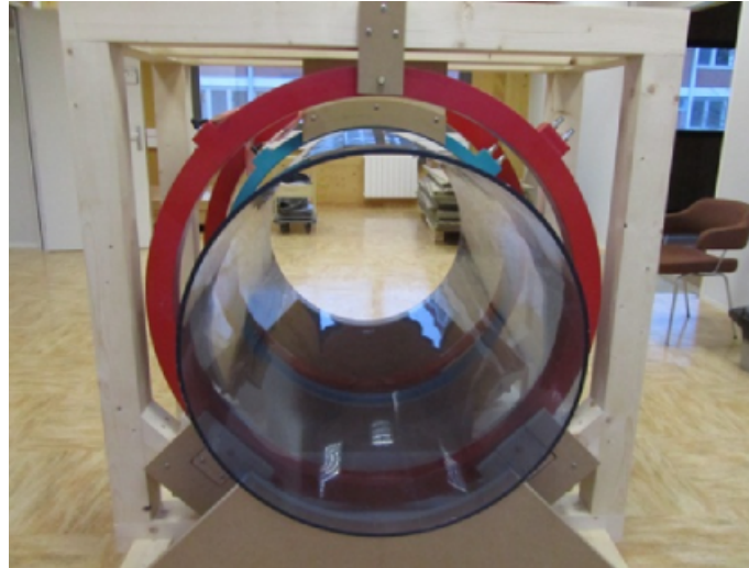
Full-head setup for MRI at very low field
