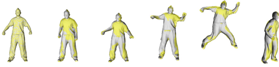
Figure 6: Optimisation of both pose and deformation. The tracking (gray) is overlaid over the target (yellow).
