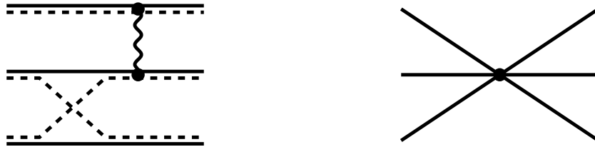
Figure 3.8: Graphical representation of a process involving three intersubband excitations (left). A first pair interact through direct Coulomb interaction. A second pair then exchange their holes. Because the diagram is connected, this interaction cannot be separated into one- and two-body effective interactions. It is, thus, an effective three-body interaction between bosonized excitations (right). Because it involves two 1/n_{QW}N_{el} contributions, it is of order (1/n_{QW}N_{el})^2 . This can be generalized to higher order process, provided the graph is connected.
