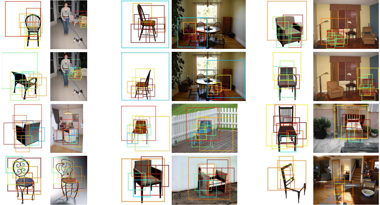
Figure 3.8: The output alignments. Matched parts are colored based on their detection confidence (warmer colors are more confident).
