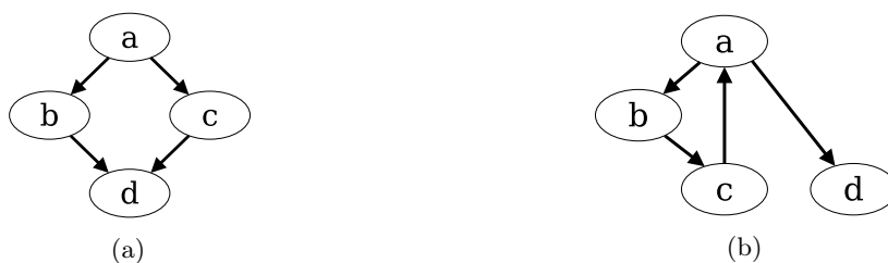
Figure 5.4: Example CFGs to illustrate postdominance and control dependencies. In both CFGs, vertex a controls vertices b and c , but not d . The first CFG represents an if statement, while the second one represents a while loop.
