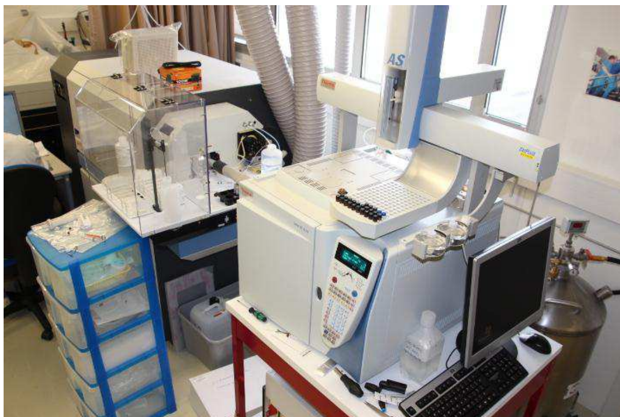
Figure 10. Picture of the GC-HR-ICPMS equipment at GET. Courtesy of J. Sonke.
