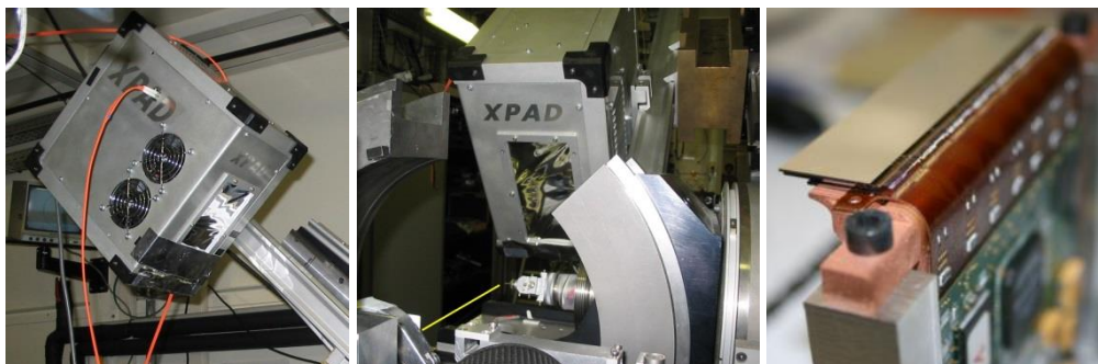
FIG. C.15: Side view (left), front view (middle) and one module (right) of the XPAD3 detector. Each module consists of 7 XPAD3 chips of 80x120 pixels. Source: D2AM website.
