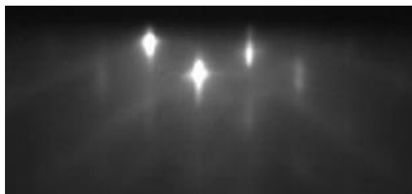
Figure 4-19: 1\times 1 RHEED pattern of the as-prepared Si (001) surface.
