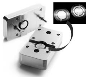
Figure 2.15 Flow cell from the Q-Sense system presented with an AT-Cut quartz crystal coated with gold
