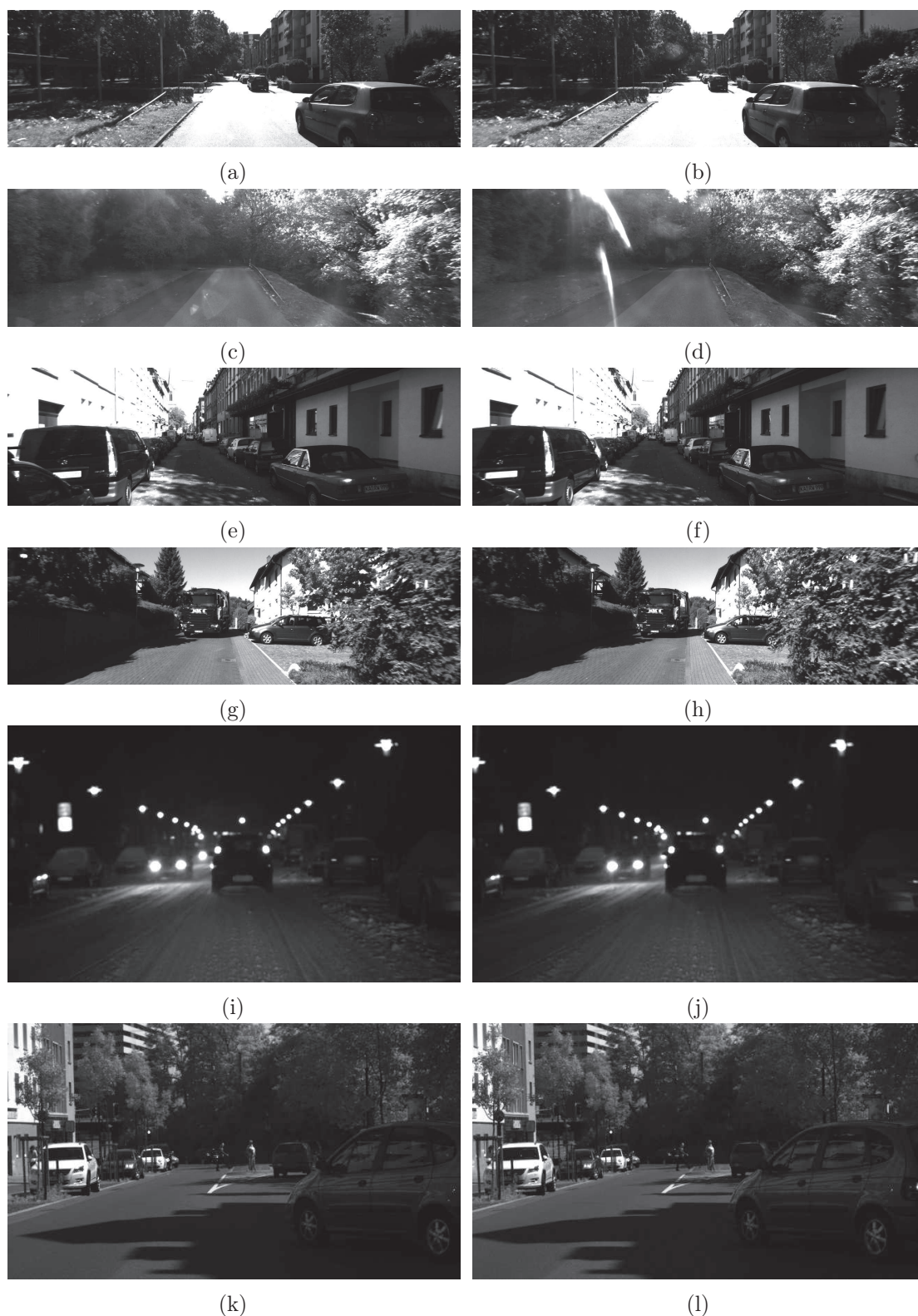
Figure 4.5: Challenging situations in stereo vision. The images a)-h) are extracted from the KITTI dataset[57], while the images i)-l) from HCI/Bosh Challenge [95]. The left column represents the left image from a stereo pair, and the right column the corresponding right image.: a)-b) Textureless area on the road caused by sun reflection; c)-d) Sun glare on the windshield produces artefacts; e)-f) "Burned" area in image where the white building continues with the sky region caused by high contrast between two areas of the image; g)-h) Road tiles produce a repetitive pattern in the images; i)-j) Night images provide fewer information; k)-l) Reflective surfaces will often produce inaccurate disparity maps
