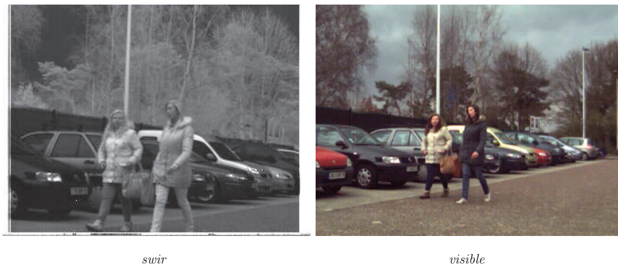
Figure 3.2: Images acquired outdoor: SWIR and visible bandwidths highlight similar features both for pedestrian and background.
