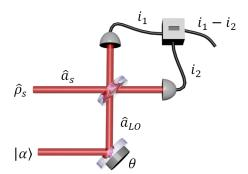
**Figure 2.5:** Homodyne detection. The measured beam is mixed with a bright coherent state called *local oscillator* on a 50:50 beam-splitter. The two outputs are measured with two photodiodes. The resulting photocurrents are subtracted and provide an output signal proportional to a quadrature measurement amplified by the amplitude of the local oscillator. Most of the time, the phase of the quadrature is adjusted with a PZT on the path of the local oscillator.
