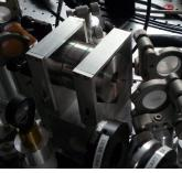
**Figure 3.1:** Scheme and picture of the  $\mu$ Cavity. The length of the cavity is adjusted with the help of ormolu of 0.2 mm (chrysocale in french).
