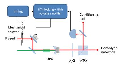
**Figure 8.7:** A weak IR beam is injected into the OPO (seed) and measured by tapping a small part of it on the conditioning path. The seed is lock in phase with the pump by using the effect of amplification (parametric gain) as the amplitude depends on the relative phase between the pump and the seed. A feed-back on a PZT changes the phase of the seed relatively to the pump. The seed has thus the same phase as the state from the output of the OPO.
