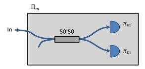
**Figure 2.3:** The measured beam is sent to a 50:50 beam-splitter with two single-photon detector connected at each output. These two detectors have the POVM element  $\hat{\pi}_m$  and  $\hat{\pi}_{m'}$ . This device can be seen as a single detector with POVM elements  $\hat{\Pi}_m$ .
