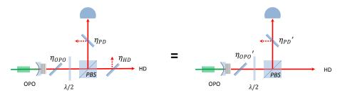
**Figure 4.2:** Loss model of the experiment. We consider a perfect OPO, single-photon detector, (PD) and homodyne detection (HD). The limited efficiency of each is modeled by fictitious beam-splitters. Because the losses of the conditioning part are higher than the homodyne detection, we can consider a model (to simplify the calculation) where only the OPO and the conditioning path are not perfect.
