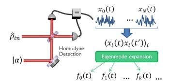
Figure 6.4: (color online). Schematic sketch. The propagating quantum state  $\hat{\rho}_{in}$  is measured by homodyne detection with a continuous-wave local oscillator. The reported method consists in accessing the optimal temporal mode via a multimode analysis using eigenfunction expansion of the autocorrelation function  $\langle x(t)x(t')\rangle$ .
