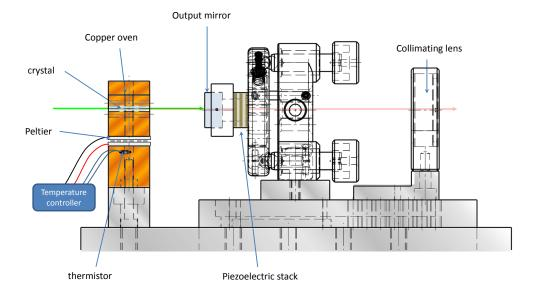
**Figure 3.6:** OPO layout. The non-linear crystal is inserted in a oven made of copper. The temperature is controlled thanks a thermistor feedback to a Peltier element. The output mirror is handled in a plastic mount glued on a piezo itself placed in a high stability mirror mount. A lens is placed right after in order to collimate the beam to a size of almost 1 mm.
