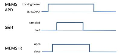
**Figure 4.6:** Some small delays are used to adjust the order of each element to avoid some unexpected behavior. The APD is disconnected prior to any locking step. Then the locking beam is send to the cavity. The size of the cavity is thus adjusted within a short time by releasing the proportional-integrate.
