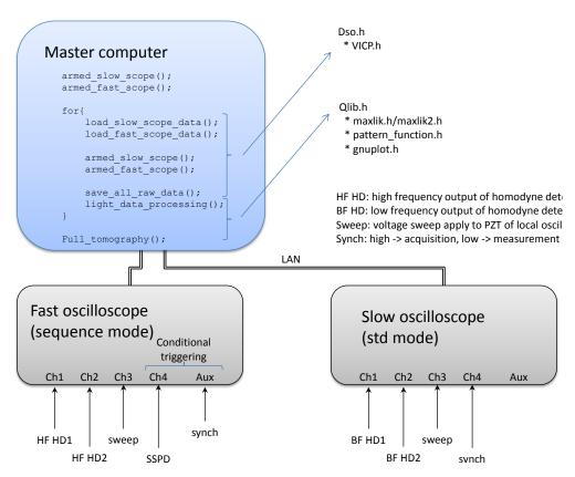
Figure 6.2: Acquisition setup for two-mode tomography (cf chapter 8)
