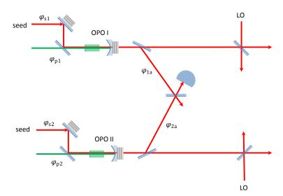
Figure 8.6: Locking of the relative phases.
