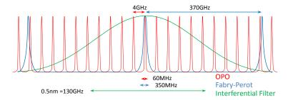
**Figure 4.4:** Conditioning path. The frequency-degenerate mode is selected by two filtering stages, first a narrow interferential filter then a Fabry-Perot cavity with a bandwidth broader than the OPO cavity bandwidth and a free spectral range bigger than the bandwidth of the interferential filter.
