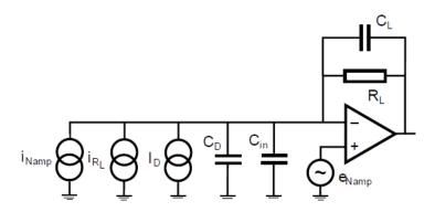
Figure 2.2: Electrical noise of the homodyne detection.
