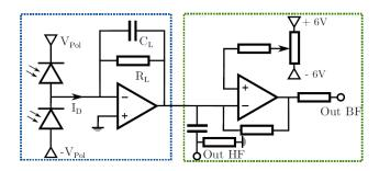
Figure 2.1: Electrical scheme of the homodyne detection.
