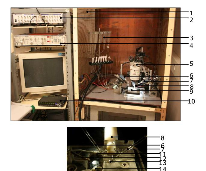
Figure 49. The classical (manual) setup for TEVC experiments [Channels Group].
