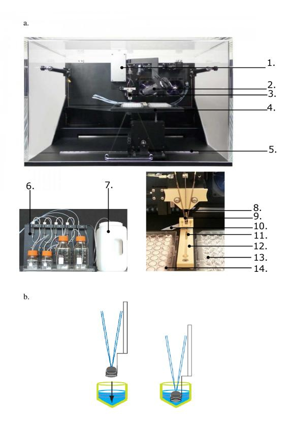
**Figure 50. An automated setup for TEVC experiments.** a) HiClamp Robot <sup>[Channels Group]</sup>. b) Motion of the basked with situated oocyte into tested solution [http://www.multichannelsystems.com].
