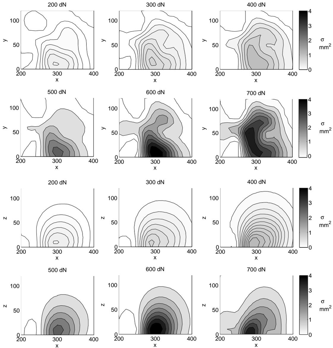
Figure 8.5: Inversion results for different loads in the  $xy$  plane and a cut in the  $xz$  plane (depth) for the concrete block with a pre-existing crack of 50 mm evaluated at  $100 \mu s$  in the coda.
