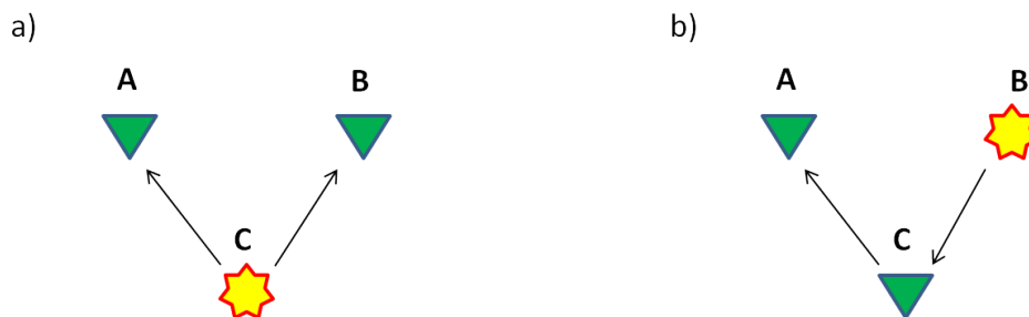
Figure 3.2: Illustration of the principle of time reversal. a) C emits a signal that is registered by A and B . b) B emits a signal that is received by C . C inverts the signal and re-emits it. A records the signal.
