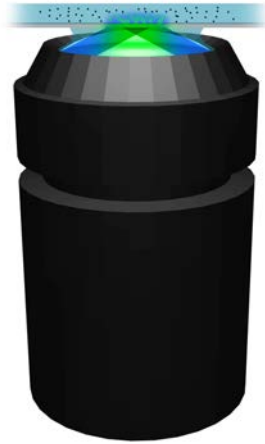
Figure 2.2: Total internal reflection of laser beam on the interface of glass slide and experimental liquid.
