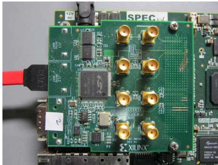
FIGURE 5.27: XM104 FMC board
