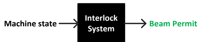
FIGURE 4.1: Interlock System functional black box
