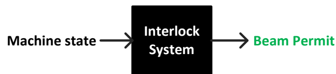
FIGURE 4.1: Interlock System functional black box
