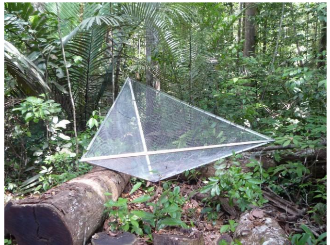
Fig. 3. Picture of the trihedral reflector.
