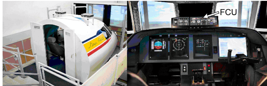
Figure 4.2: The ISAE 3-axis flight simulator. Left: outside view of the cabin. Right: cockpit view, the arrow indicates the position of the Flight Control Unit (FCU) dedicated to autopilot programming (heading, speed, altitude and vertical speed selection). The participants flew the aircraft from the left seat.
